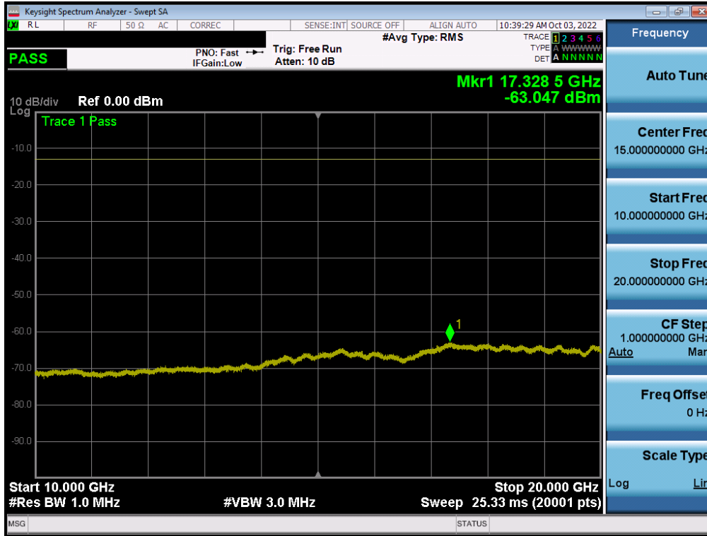
Plot 7-189. Conducted Spurious Plot (LTE Band 66/4 - 20MHz QPSK - 1 RB - Low Channel – Ant F)
