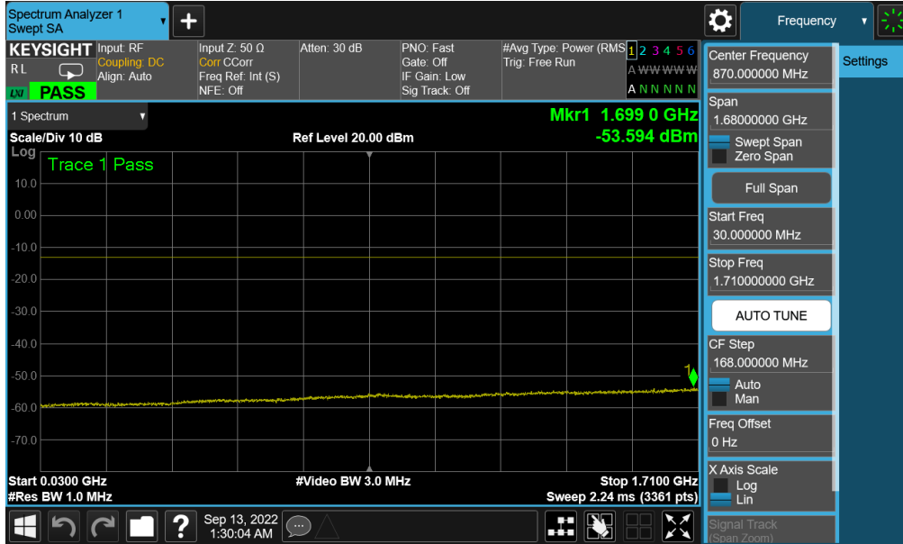
Plot 7-163. Conducted Spurious Plot (LTE Band 66/4 - 20MHz QPSK - 1 RB - High Channel – Ant A)
