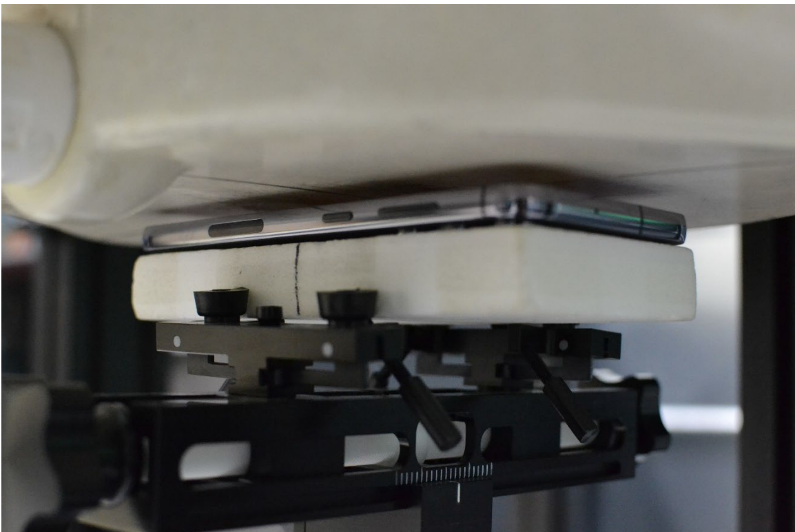
SAR Test Setup Photo 10 – Phablet, Front Side at 7mm
