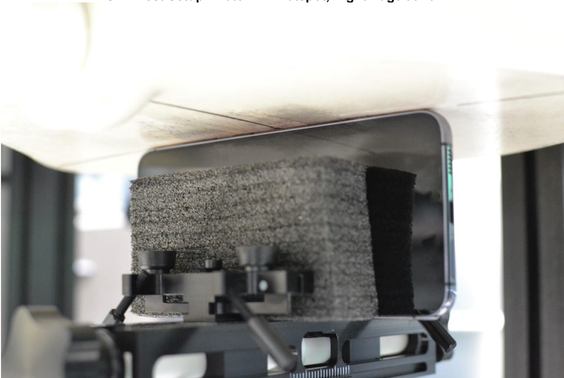
SAR Test Setup Photo 18 – Phablet, Right Edge at 0mm
