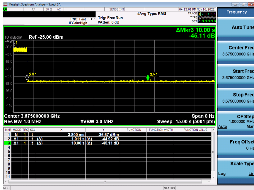
Plot 7-185. Run#2 End User Device Discontinues Operations within 10s
