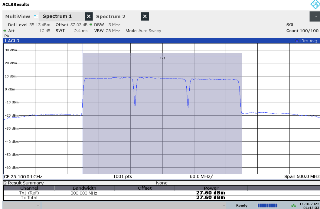
Plot 7-82. Ant 2 EIRP Plot (Band n258-R2 – 100MHz-3CC – pi/2-BPSK – High Channel)
