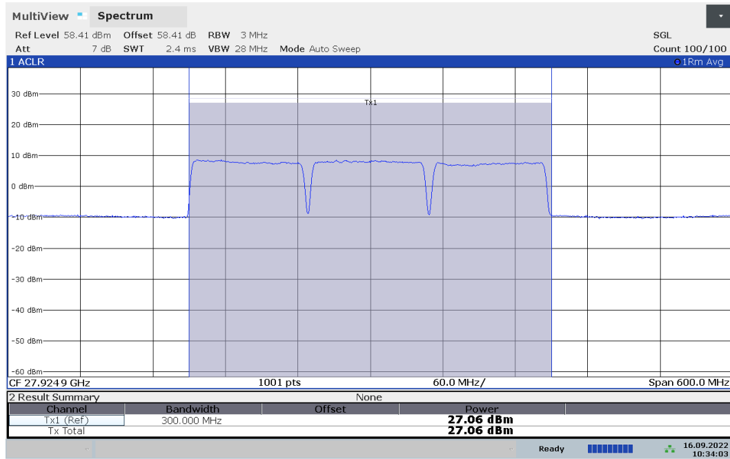
Plot 7-91. Ant 2 EIRP Plot (Band n261 – 100MHz-3CC – QPSK – Mid Channel)
