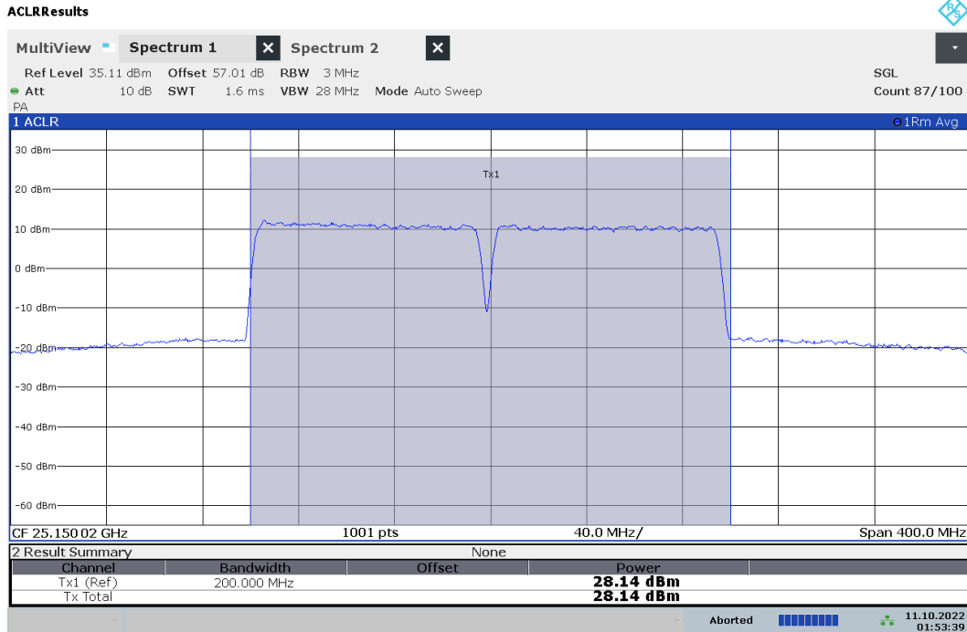
Plot 7-81. Ant 2 EIRP Plot (Band n258-R2 – 100MHz-2CC – pi/2-BPSK – High Channel)
