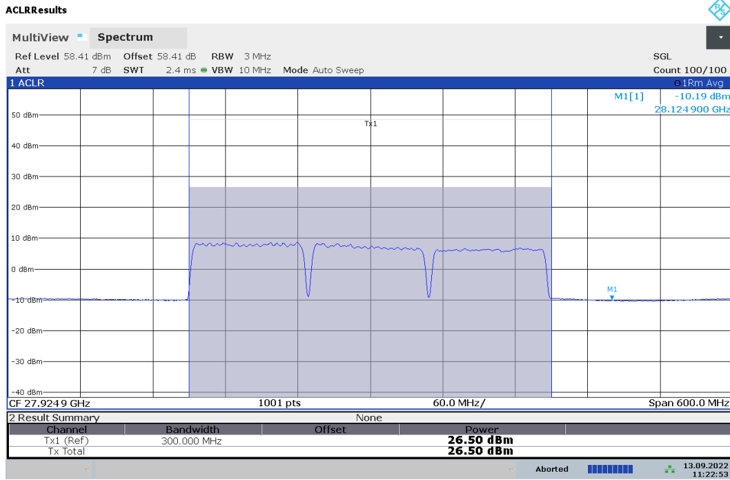
Plot 7-86. Ant 1 EIRP Plot (Band n261 – 100MHz-3CC – QPSK – Mid Channel)
