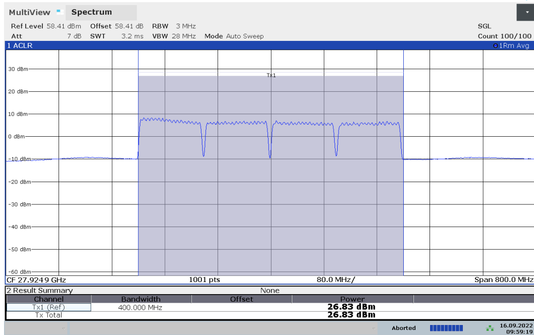
Plot 7-92. Ant 2 EIRP Plot (Band n261 – 100MHz-4CC – pi/2-BPSK – Mid Channel)
