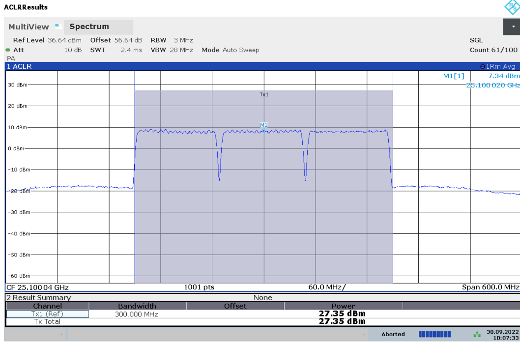
Plot 7-78. Ant 1 EIRP Plot (Band n258-R2 – 100MHz-3CC – QPSK – High Channel)
