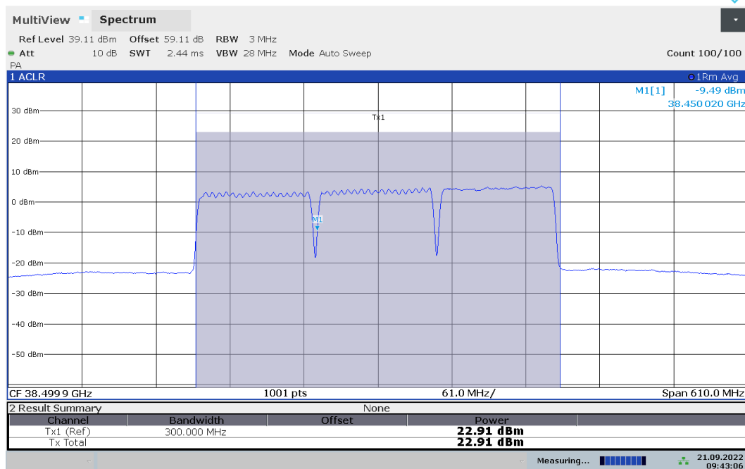
Plot 7-96. Ant 1 EIRP Plot (Band n260 – 100MHz-3CC – QPSK – Mid Channel)
