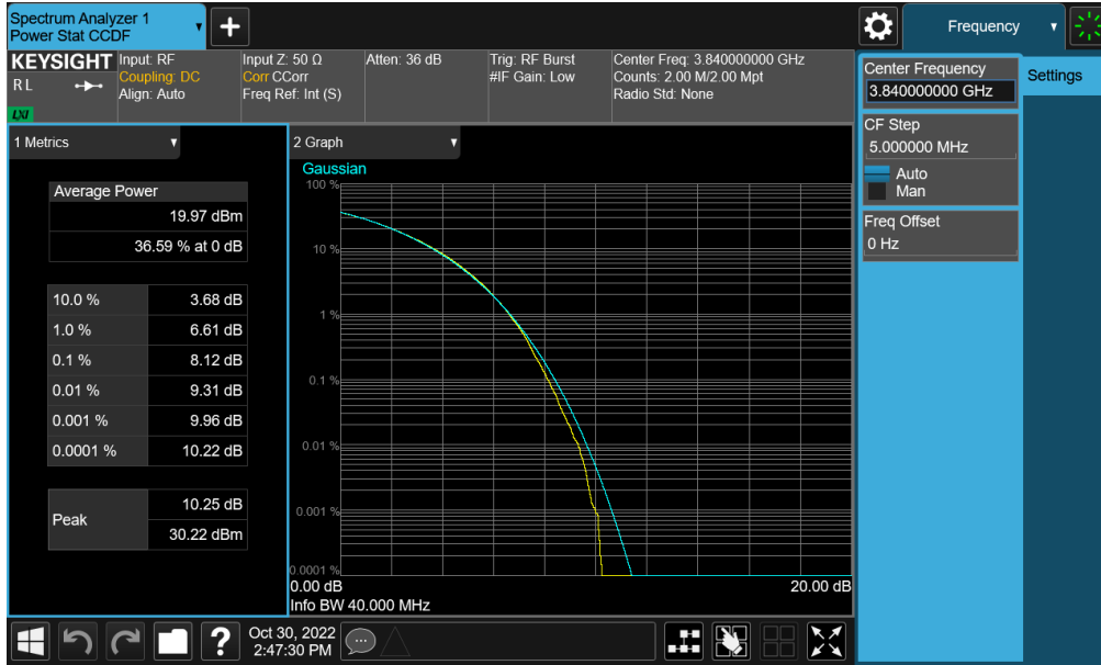
Plot 7-237. PAR Plot (NR Band n77 - C-Band – 40MHz CP-OFDM 256-QAM - Full RB)
