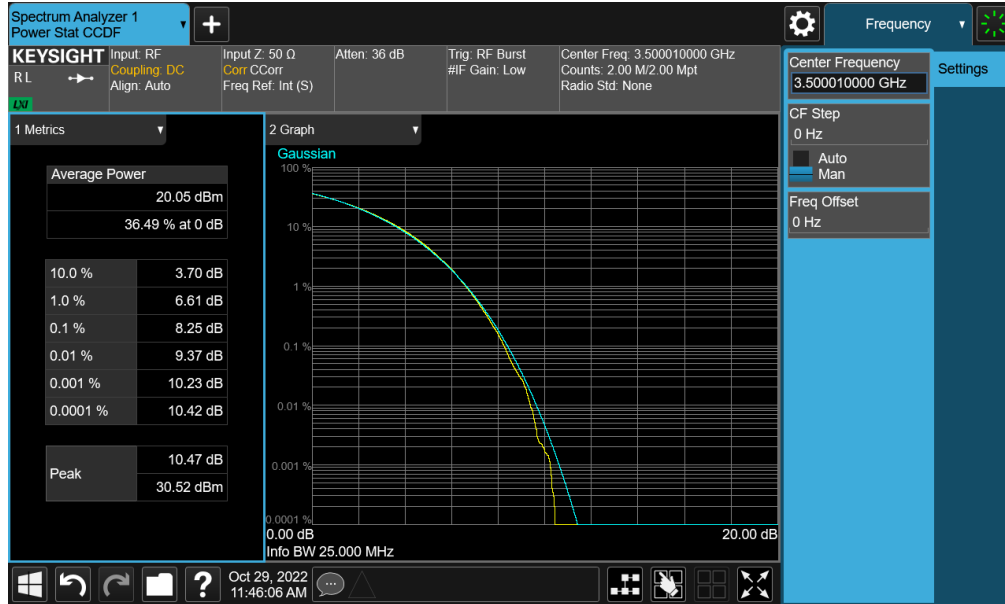
Plot 7-207. PAR Plot (NR Band n77 - DoD Band – 25MHz CP-OFDM 256-QAM - Full RB)
