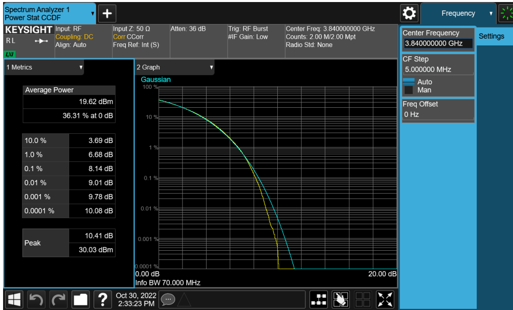
Plot 7-228. PAR Plot (NR Band n77 - C-Band – 70MHz CP-OFDM 256-QAM - Full RB)
