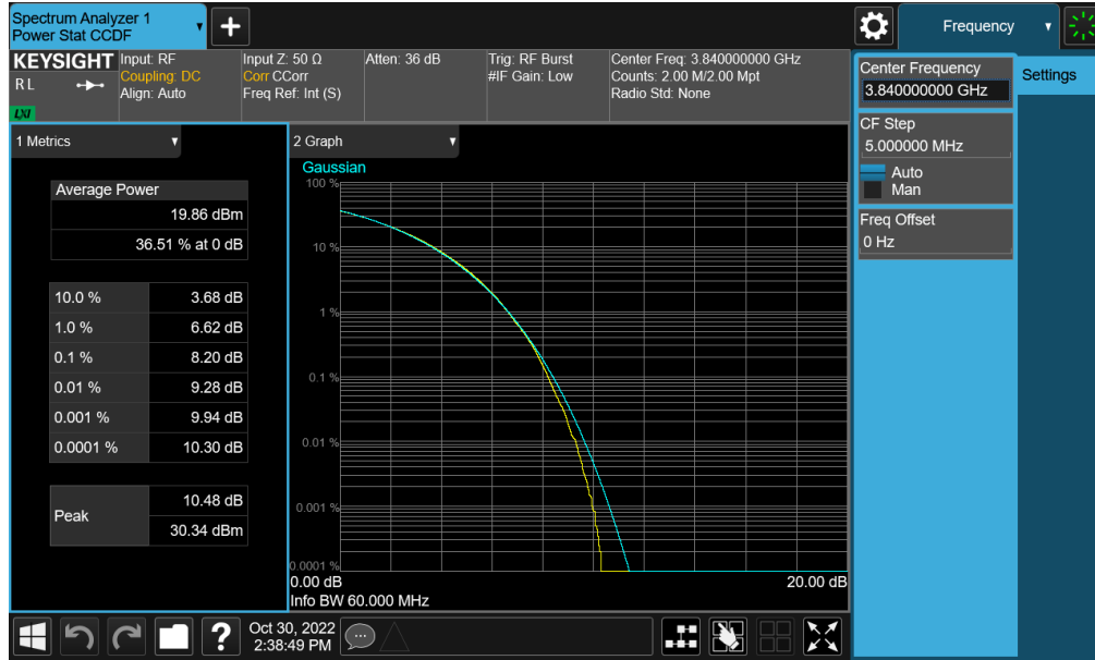
Plot 7-231. PAR Plot (NR Band n77 - C-Band – 60MHz CP-OFDM 256-QAM - Full RB)
