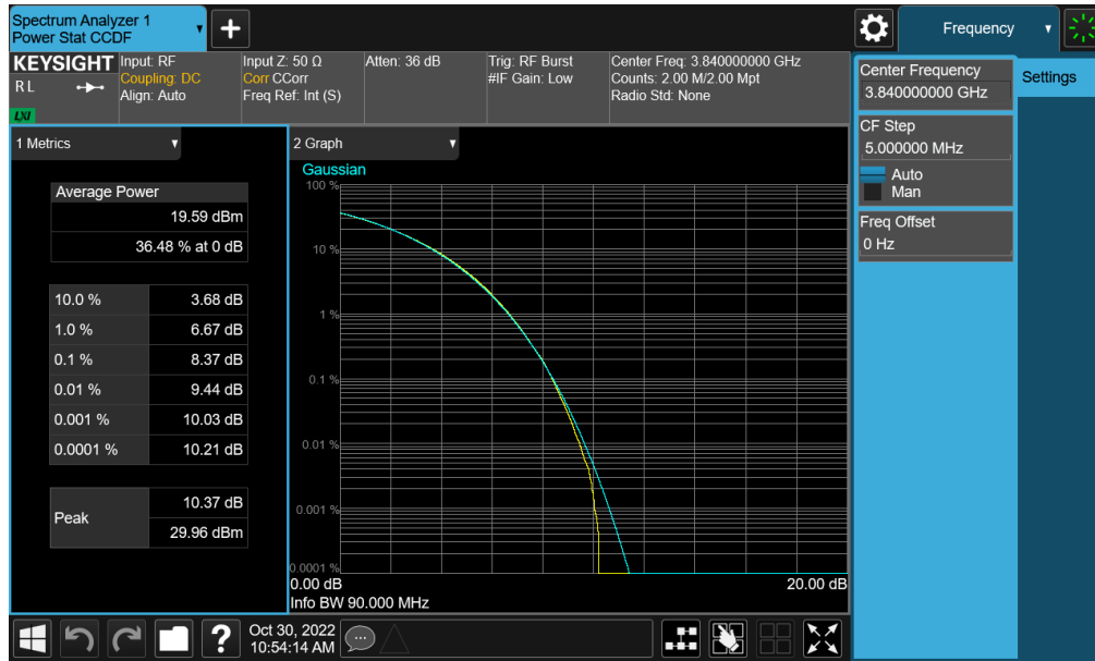
Plot 7-222. PAR Plot (NR Band n77 - C-Band - 90MHz CP-OFDM 256-QAM - Full RB)
