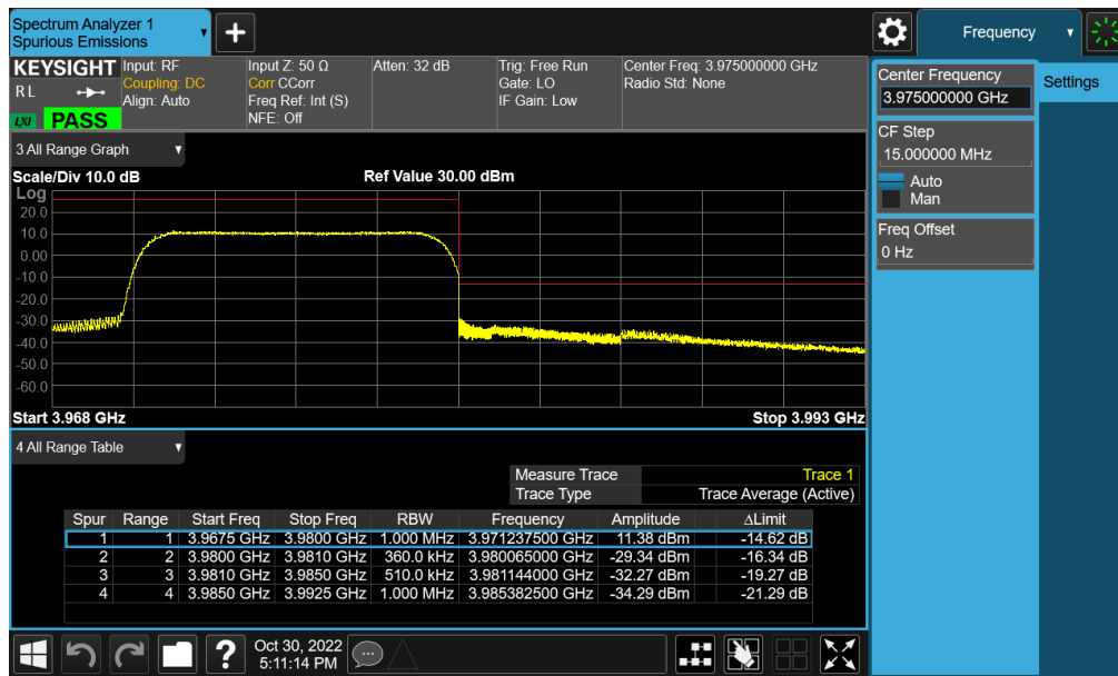
Plot 7-174. Upper ACP Plot (NR Band n77 - C-Band – 10MHz DFT-s-OFDM \pi/2 BPSK – Full RB - SRS-1)
