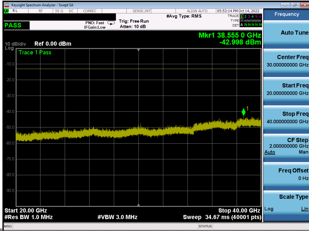
Plot 7-114. Conducted Spurious Plot (NR Band n77 - C-Band – 100MHz QPSK - RB Size 1, RB Offset 0 - Low Channel - SRS-4)
