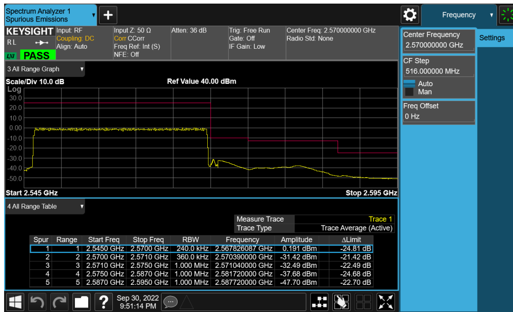
Plot 7-422. Upper Band Edge Plot (NR Band n7 - 25MHz CP-OFDM-QPSK – Full RB - Ant F)
