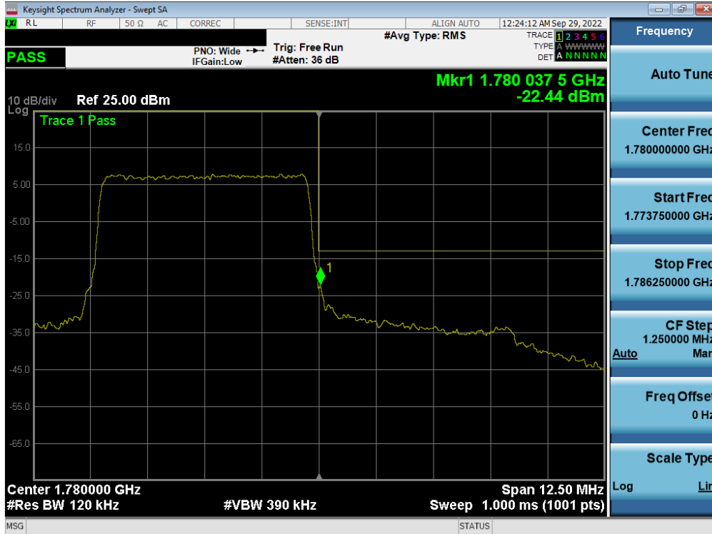
Plot 7-345. Upper Band Edge Plot (LTE Band 66 - 5MHz QPSK – Full RB - Ant F)
