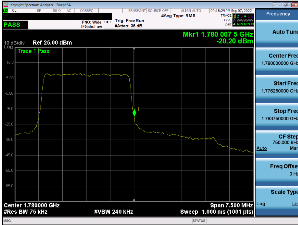
Plot 7-283. Upper Band Edge Plot (LTE Band 66 - 3MHz QPSK – Full RB - ANT A)
