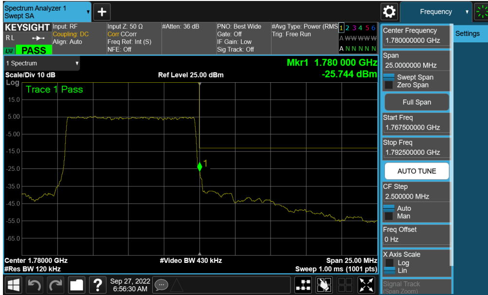
Plot 7-313. Upper Band Edge Plot (NR Band n66 – 10.0MHz - Full RB - ANT A)
