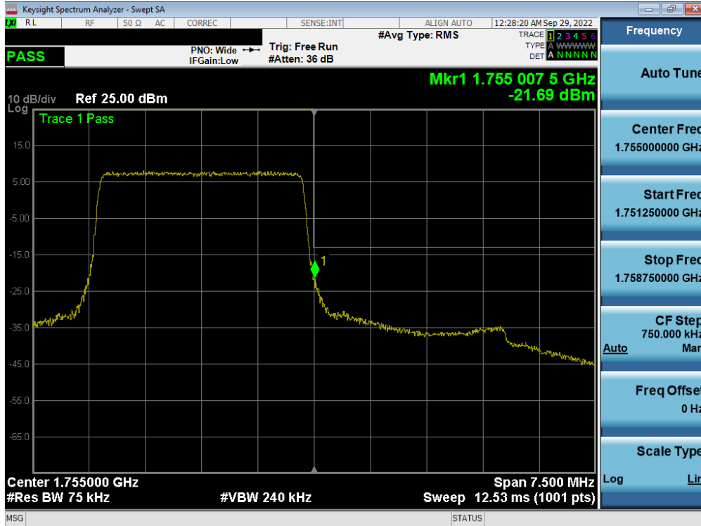
Plot 7-349. Upper Band Edge Plot (LTE Band 4 - 3MHz QPSK – Full RB - Ant F)
