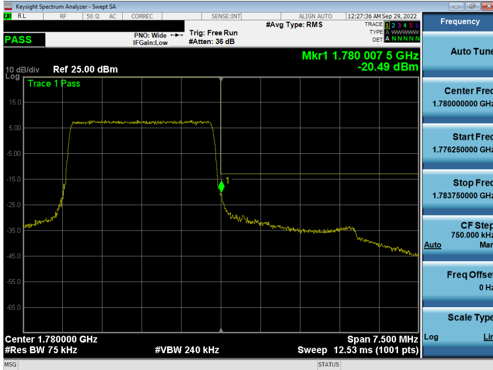
Plot 7-351. Upper Band Edge Plot (LTE Band 66 - 3MHz QPSK – Full RB - Ant F)
