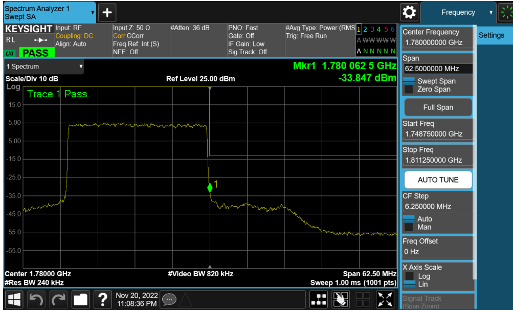
Plot 7-301. Upper Band Edge Plot (NR Band n66 – 25.0MHz - Full RB - ANT A)
