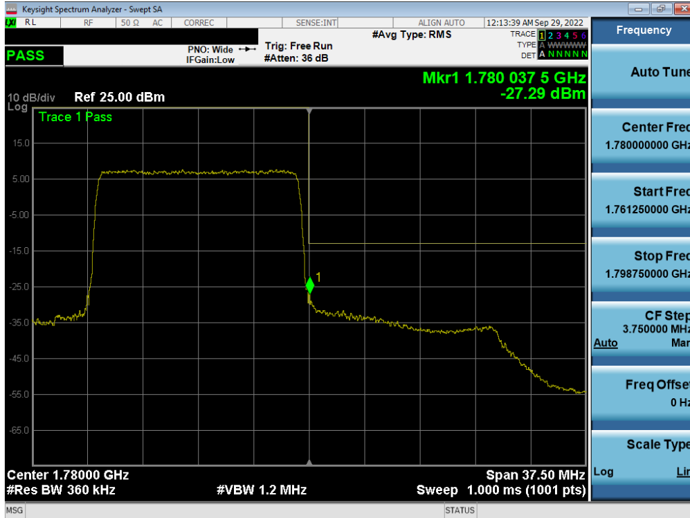
Plot 7-333. Upper Band Edge Plot (LTE Band 66 - 15MHz QPSK – Full RB - Ant F)
