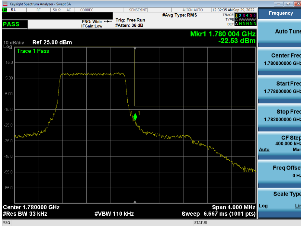
Plot 7-357. Upper Band Edge Plot (LTE Band 66 – 1.4MHz QPSK – Full RB - Ant F)
