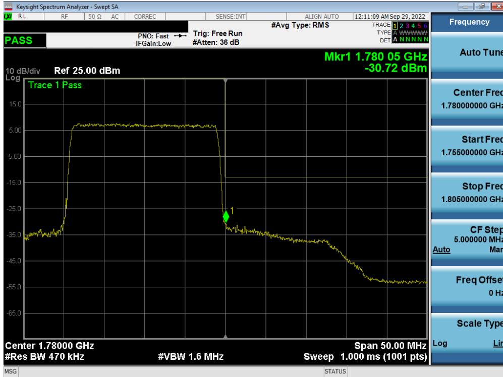
Plot 7-327. Upper Band Edge Plot (LTE Band 66 - 20MHz QPSK – Full RB - Ant F)
