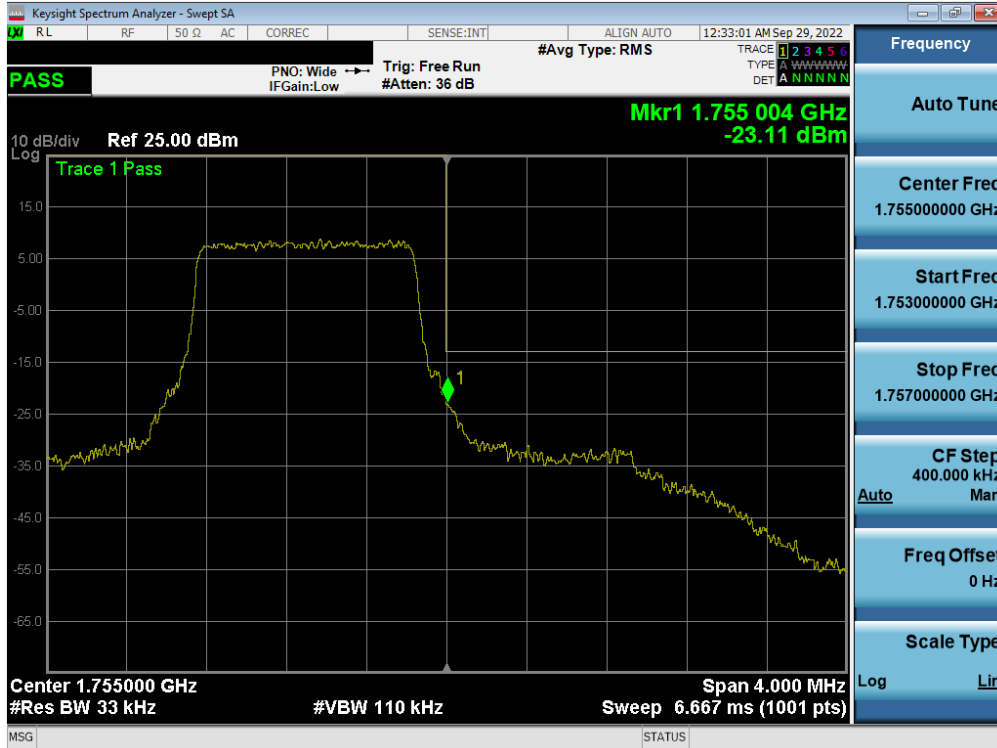
Plot 7-355. Upper Band Edge Plot (LTE Band 4 – 1.4MHz QPSK – Full RB - Ant F)
