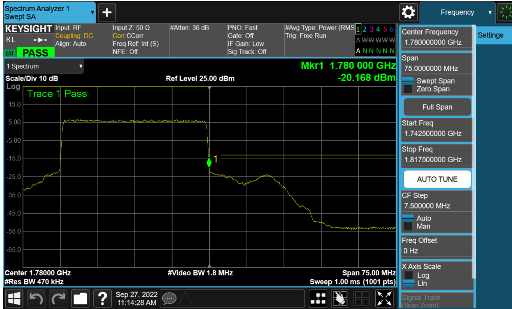
Plot 7-365. Upper Band Edge Plot (NR Band n66 – 30.0MHz - Full RB - Ant F)
