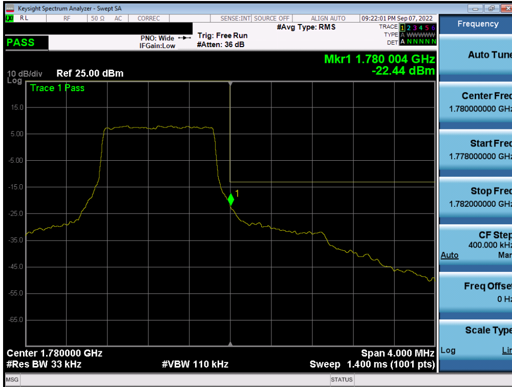
Plot 7-289. Upper Band Edge Plot (LTE Band 66 – 1.4MHz QPSK – Full RB - ANT A)
