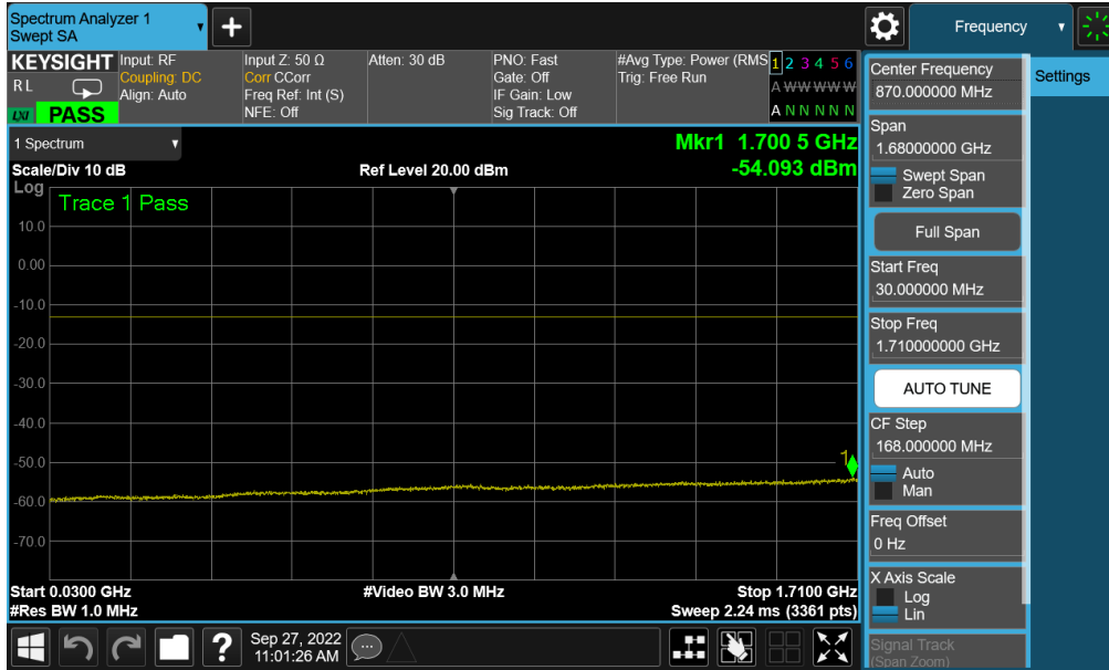
Plot 7-198. Conducted Spurious Plot (NR Band n66 - 40.0MHz - 1 RB - High Channel - Ant F)
