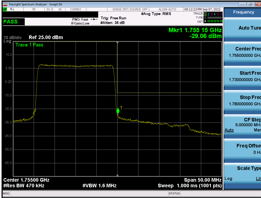
Plot 7-257. Upper Band Edge Plot (LTE Band 4 - 20MHz QPSK – Full RB - ANT A)
