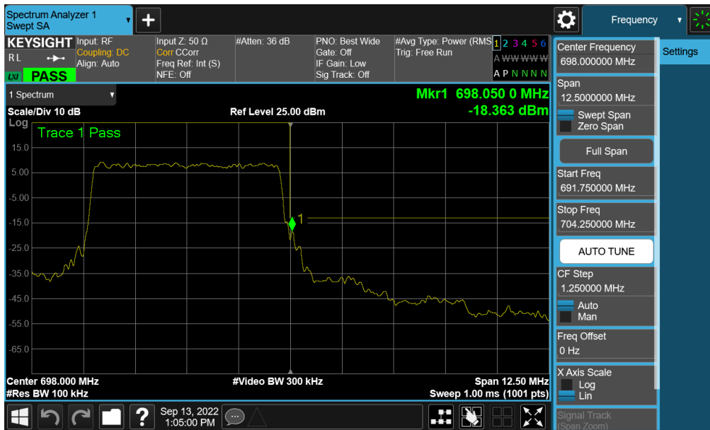
Plot 7-244. Upper Band Edge Plot (NR Band n71 – 5.0MHz - Full RB - ANT A)
