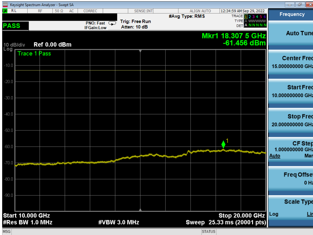
Plot 7-185. Conducted Spurious Plot (LTE Band 66/4 - 20MHz QPSK - 1 RB - Low Channel – Ant F)
