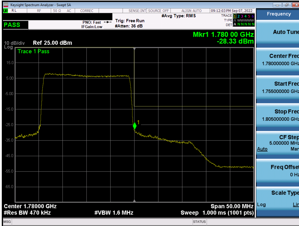
Plot 7-259. Upper Band Edge Plot (LTE Band 66 - 20MHz QPSK – Full RB - ANT A)
