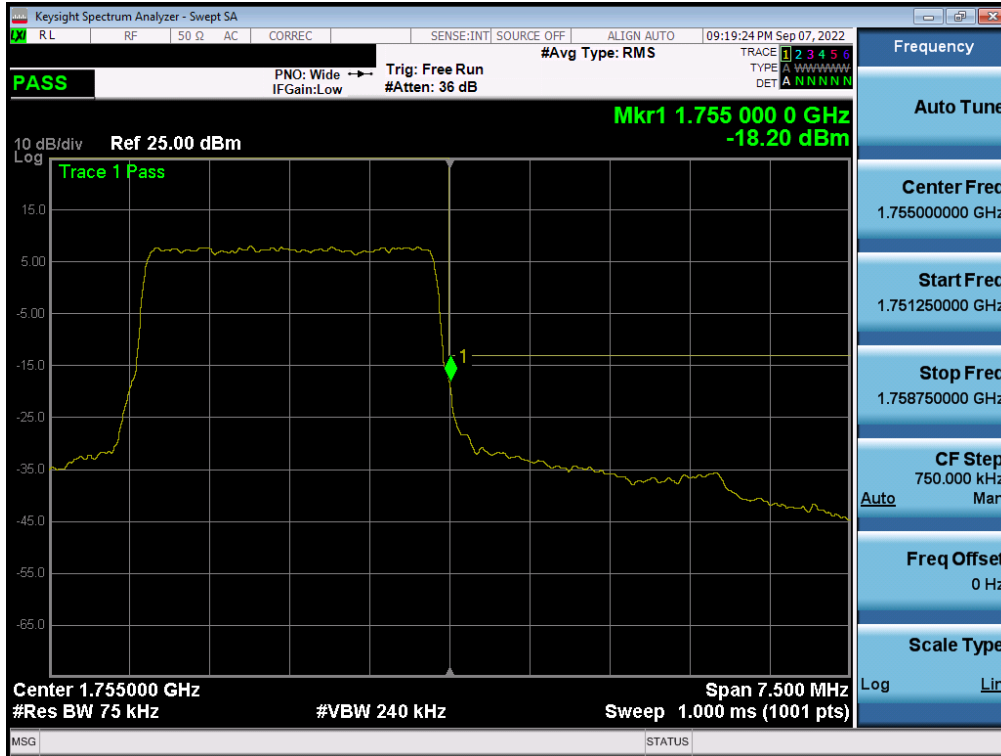
Plot 7-281. Upper Band Edge Plot (LTE Band 4 - 3MHz QPSK – Full RB - ANT A)
