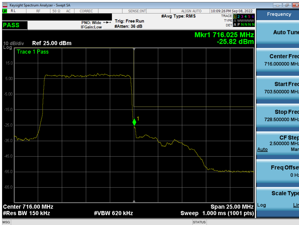
Plot 7-248. Upper Band Edge Plot (NR Band n12 – 10.0MHz - Full RB - ANT A)
