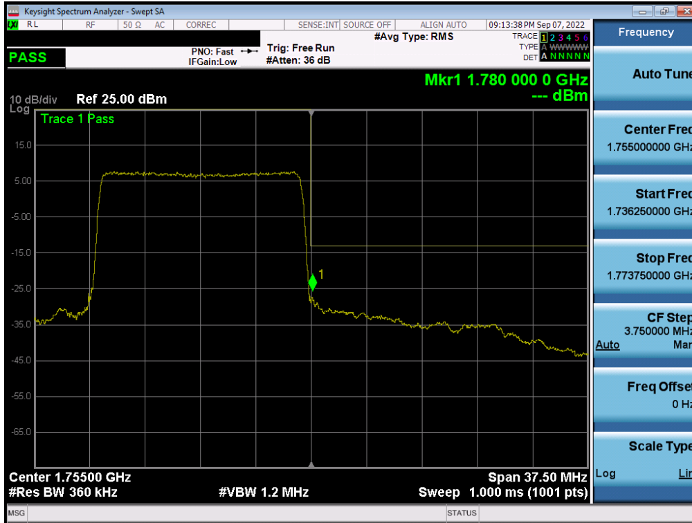
Plot 7-263. Upper Band Edge Plot (LTE Band 4 - 15MHz QPSK – Full RB - ANT A)
