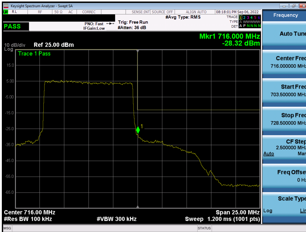
Plot 7-222. Upper Band Edge Plot (LTE Band 12 - 10MHz QPSK – Full RB - ANT A)
