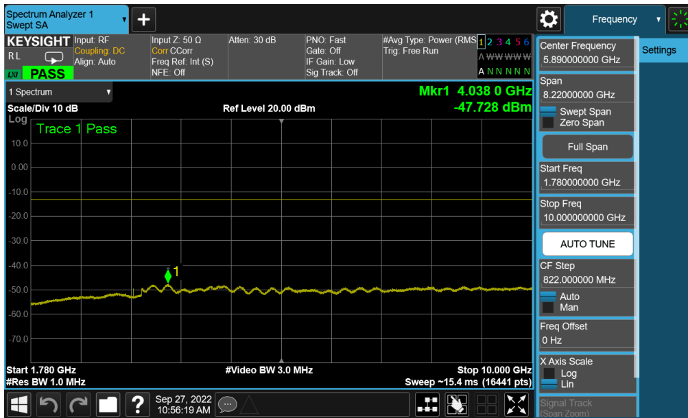
Plot 7-193. Conducted Spurious Plot (NR Band n66 - 40.0MHz - 1 RB - Low Channel - Ant F)
