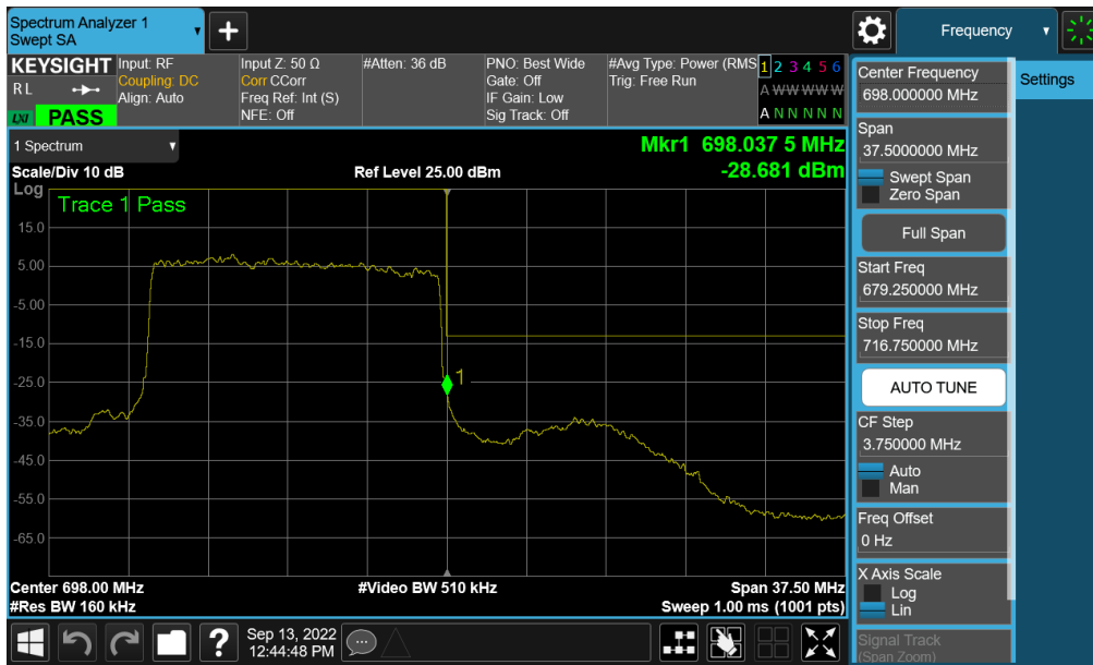
Plot 7-240. Upper Band Edge Plot (NR Band n71 – 15.0MHz - Full RB - ANT A)
