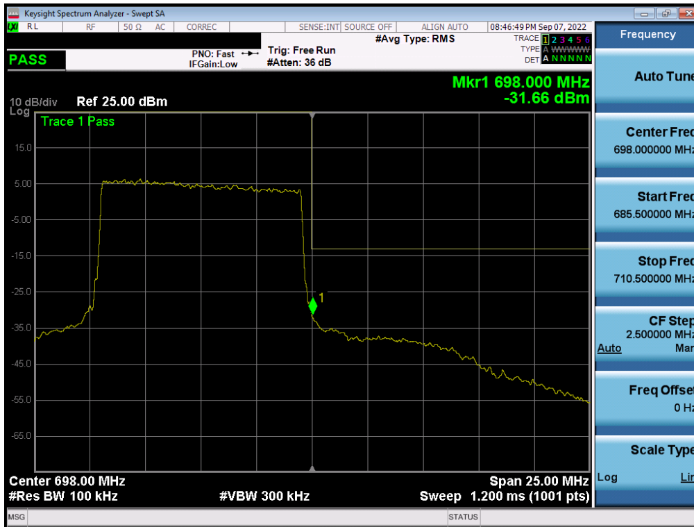
Plot 7-218. Upper Band Edge Plot (LTE Band 71 - 10MHz QPSK – Full RB - ANT A)
