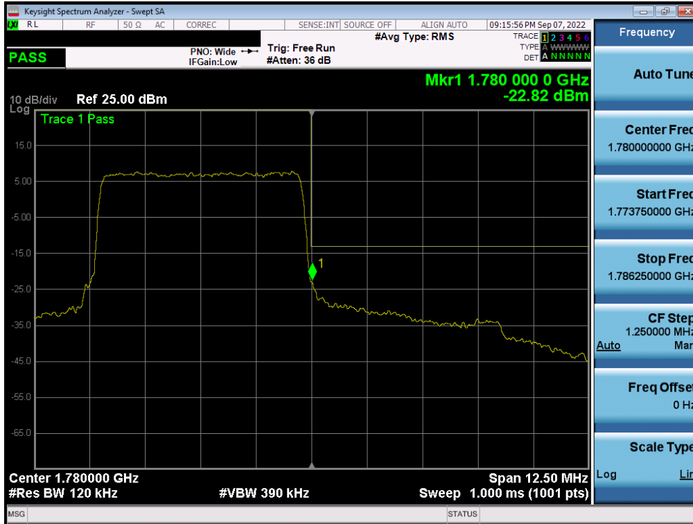
Plot 7-277. Upper Band Edge Plot (LTE Band 66 - 5MHz QPSK – Full RB - ANT A)
