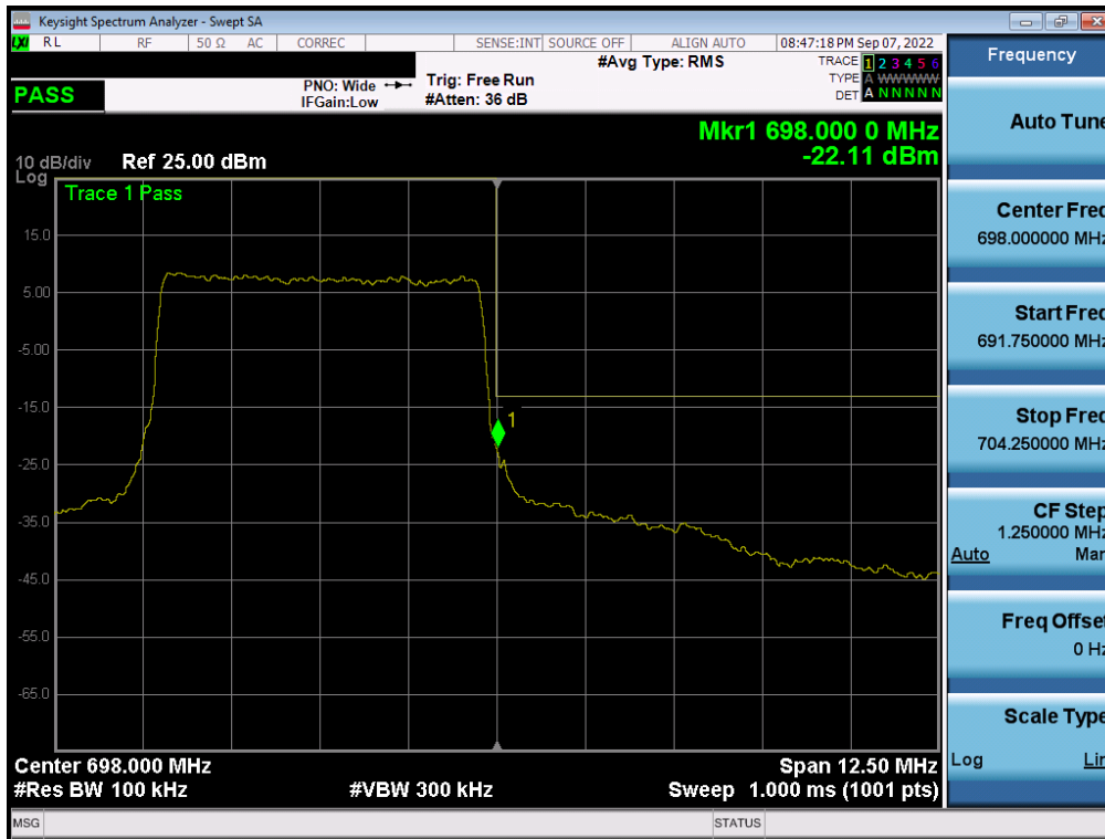
Plot 7-220. Upper Band Edge Plot (LTE Band 71 - 5MHz QPSK – Full RB - ANT A)
