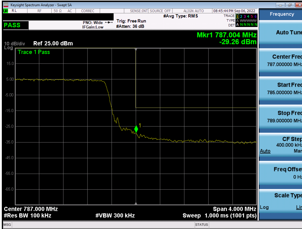
Plot 7-231. Upper Band Edge Plot (LTE Band 13 - 10MHz QPSK – Full RB - ANT A)
