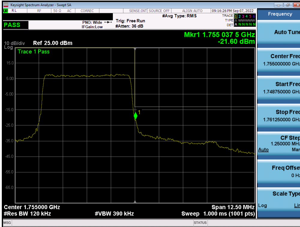
Plot 7-275. Upper Band Edge Plot (LTE Band 4 - 5MHz QPSK – Full RB - ANT A)
