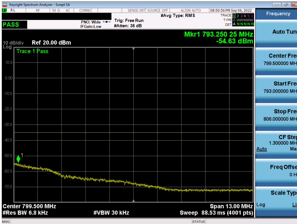
Plot 7-236. Upper Emission Mask Plot (LTE Band 13 - 5MHz QPSK – Full RB - ANT A)
