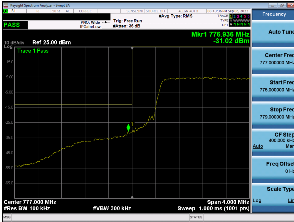
Plot 7-229. Lower Band Edge Plot (LTE Band 13 - 10MHz QPSK – Full RB - ANT A)
