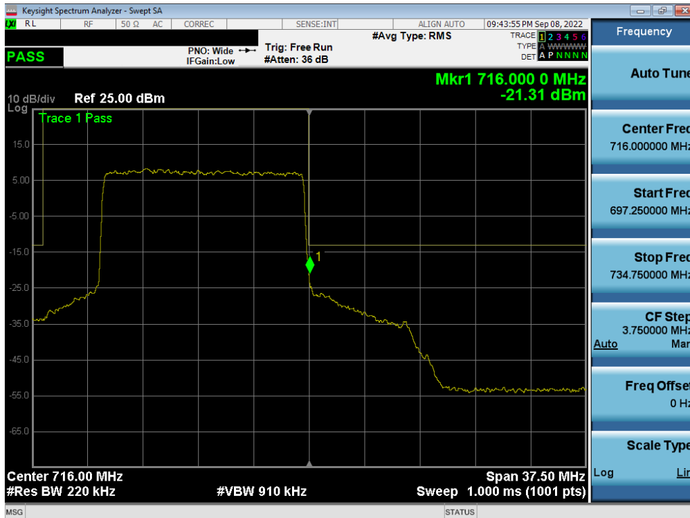
Plot 7-246. Upper Band Edge Plot (NR Band n12 – 15.0MHz - Full RB - ANT A)
