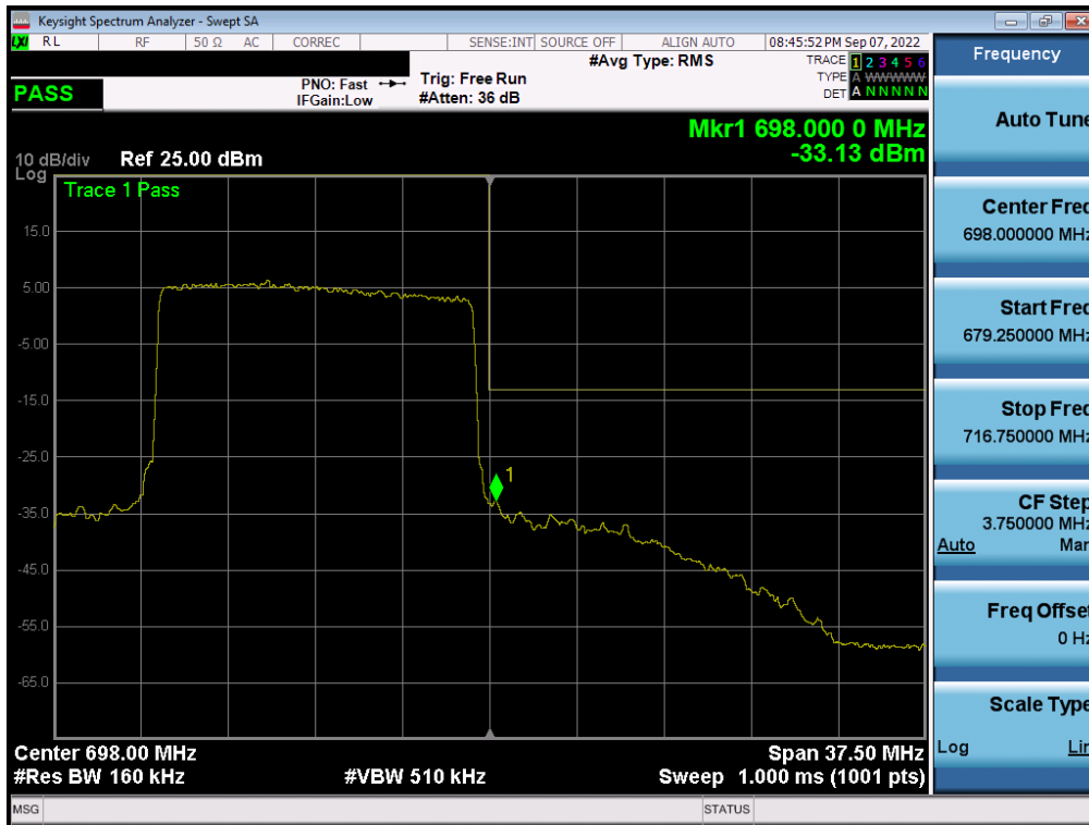
Plot 7-216. Upper Band Edge Plot (LTE Band 71 - 15MHz QPSK – Full RB - ANT A)
