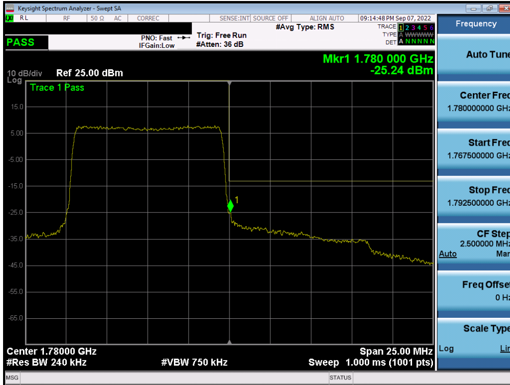
Plot 7-271. Upper Band Edge Plot (LTE Band 66 - 10MHz QPSK – Full RB - ANT A)
