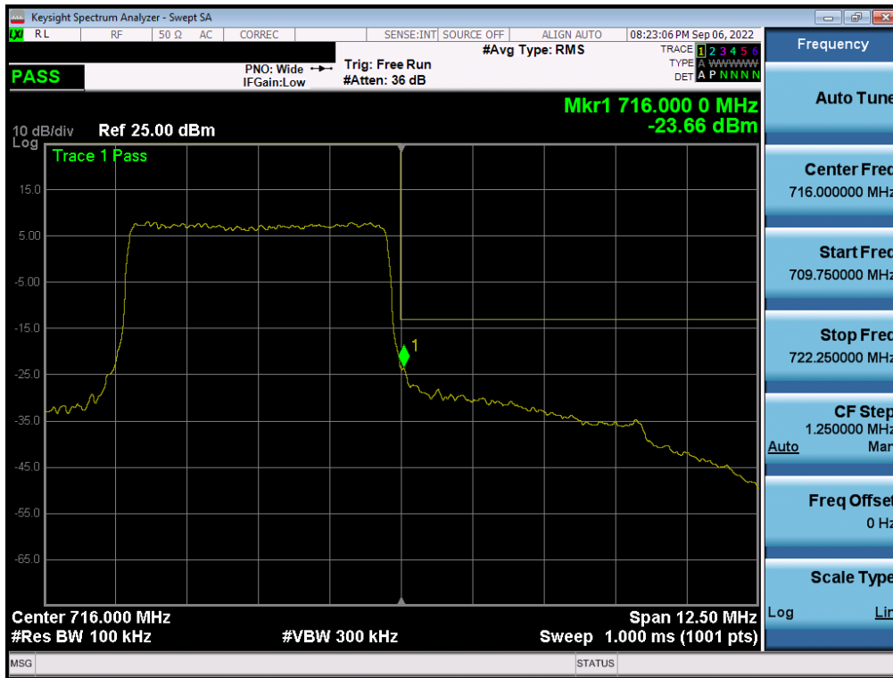
Plot 7-224. Upper Band Edge Plot (LTE Band 12 - 5MHz QPSK – Full RB - ANT A)
