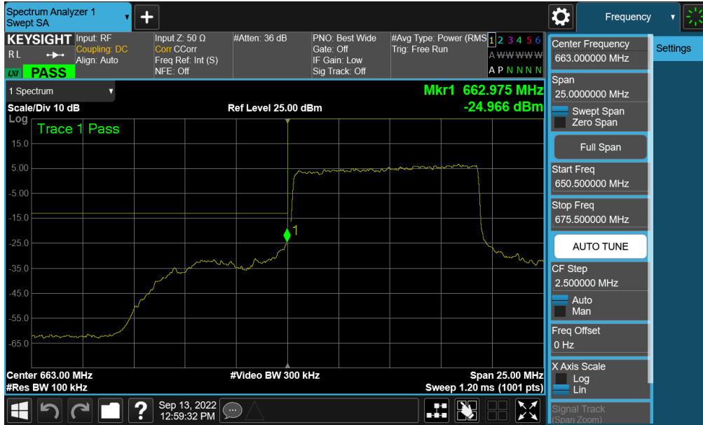
Plot 7-241. Lower Band Edge Plot (NR Band n71 – 10.0MHz - Full RB - ANT A)
