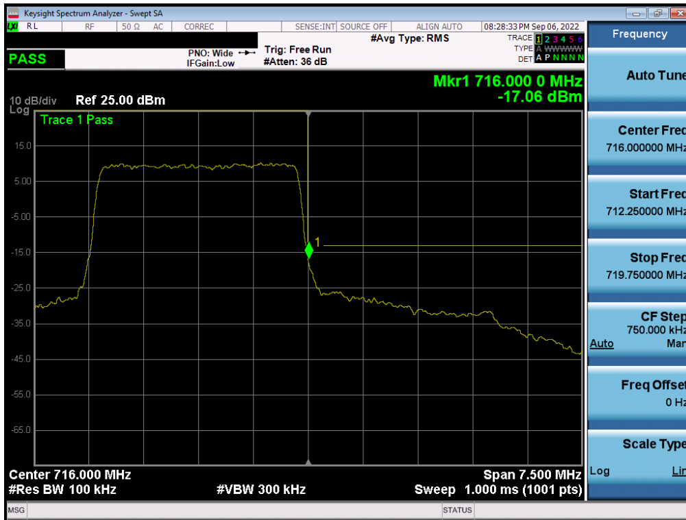
Plot 7-226. Upper Band Edge Plot (LTE Band 12 - 3MHz QPSK – Full RB - ANT A)
