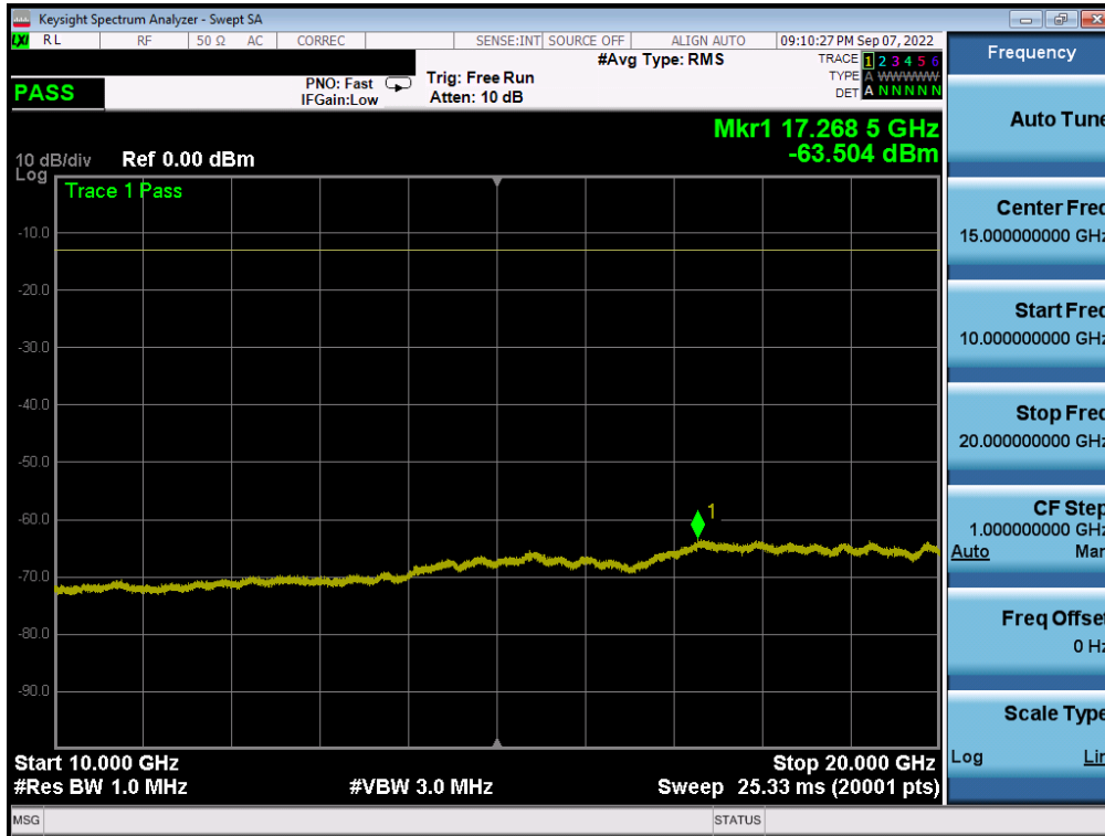
Plot 7-158. Conducted Spurious Plot (LTE Band 66/4 - 20MHz QPSK - 1 RB - Mid Channel – ANT A)
