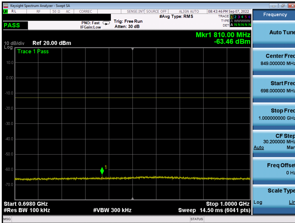
Plot 7-106. Conducted Spurious Plot (LTE Band 71 - 20MHz QPSK - 1 RB - Low Channel - ANT A)
