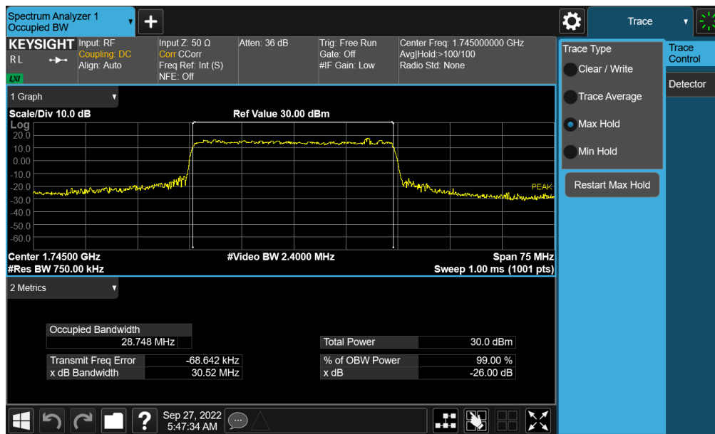
Plot 7-56. Occupied Bandwidth Plot (NR Band n66 - 30.0MHz CP-OFDM 16QAM - Full RB – ANT A)
