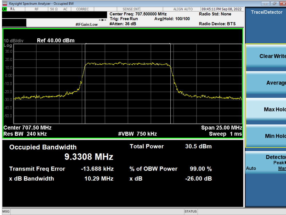
Plot 7-33. Occupied Bandwidth Plot (NR Band n12 - 10MHz CP-OFDM QPSK - Full RB – ANT A)
