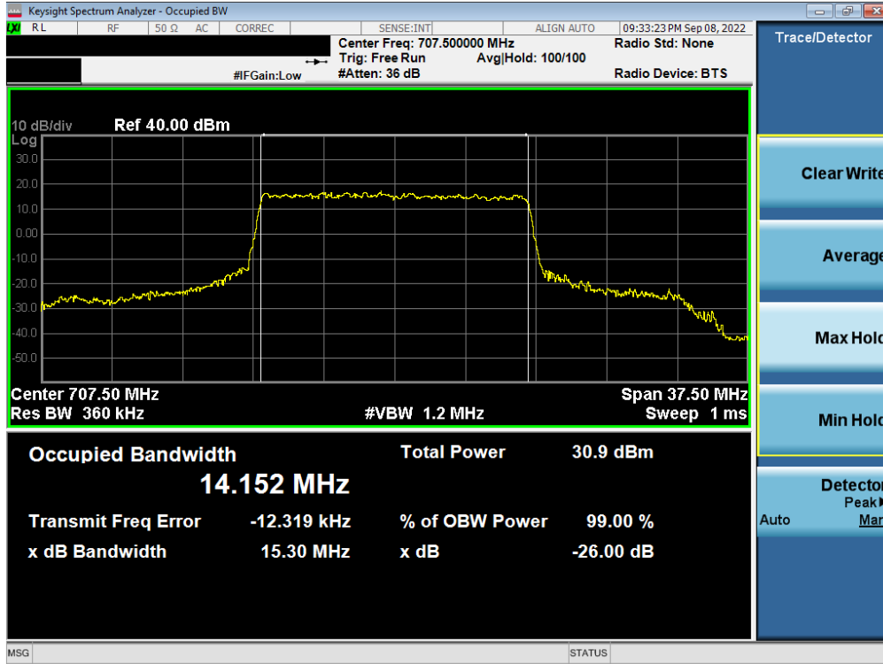
Plot 7-31. Occupied Bandwidth Plot (NR Band n12 - 15MHz CP-OFDM 16-QAM - Full RB – ANT A)
