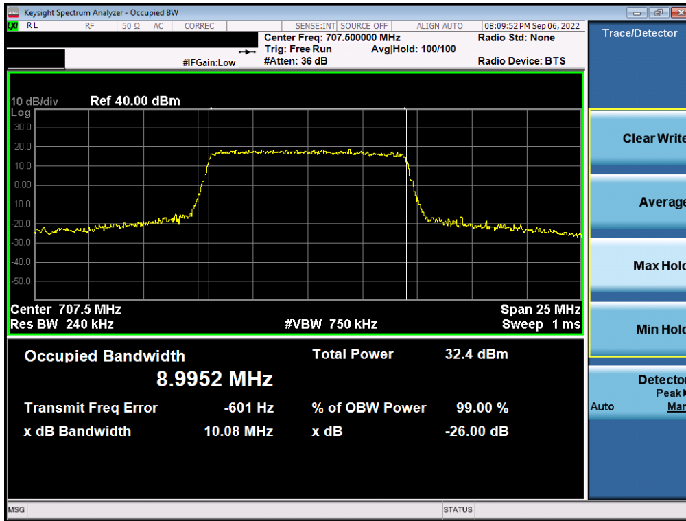
Plot 7-9. Occupied Bandwidth Plot (LTE Band 12 - 10MHz QPSK - Full RB – ANT A)
