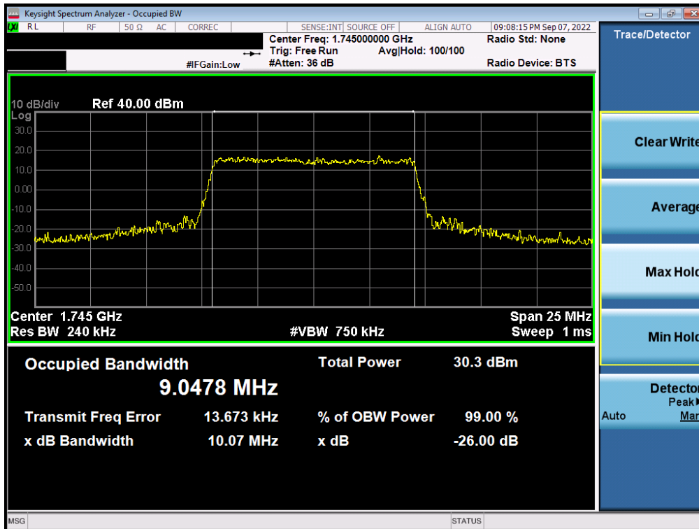
Plot 7-44. Occupied Bandwidth Plot (LTE Band 66/4 - 10MHz 16-QAM - Full RB - ANT A)
