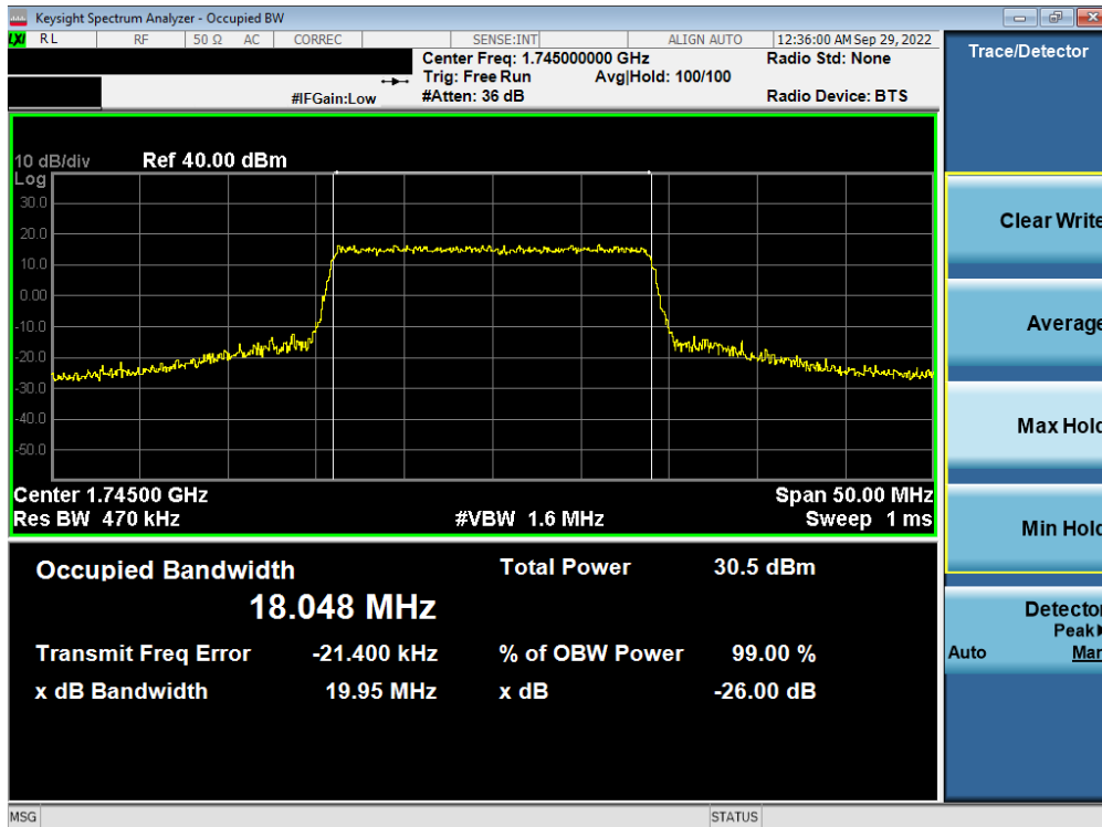
Plot 7-73. Occupied Bandwidth Plot (LTE Band 66/4 - 20MHz 16-QAM - Full RB - Ant F)
