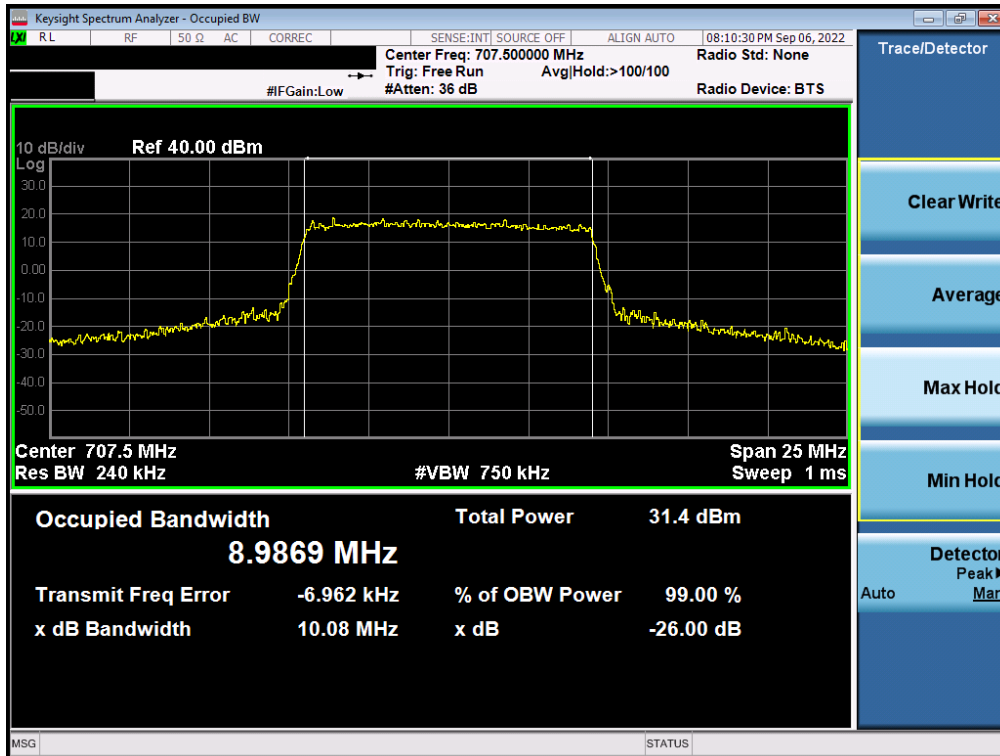
Plot 7-10. Occupied Bandwidth Plot (LTE Band 12 - 10MHz 16-QAM - Full RB – ANT A)
