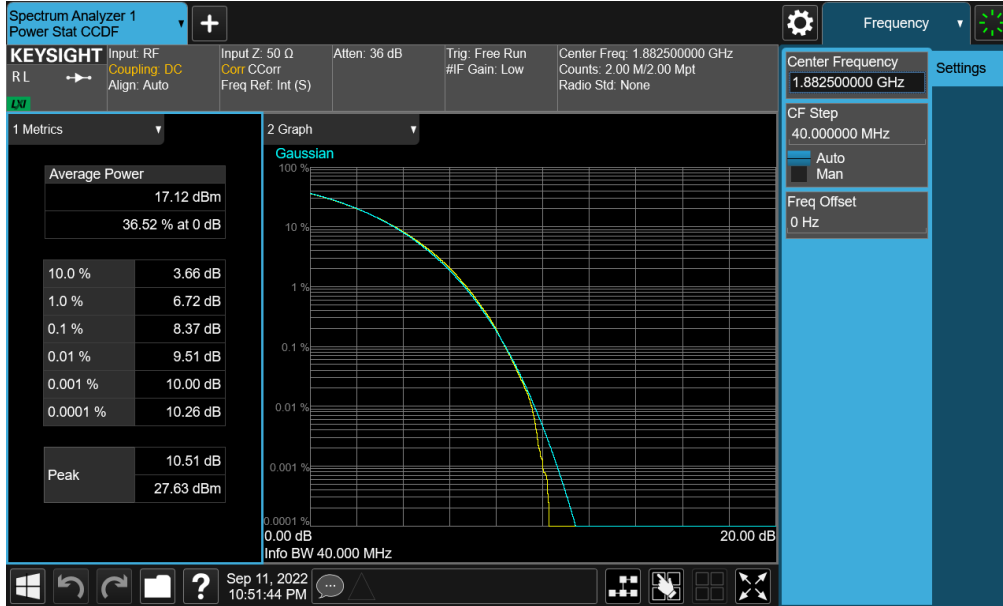
Plot 7-288. PAR Plot (NR Band n25 - 40.0MHz CP-OFDM 256-QAM - Full RB - Ant A)
