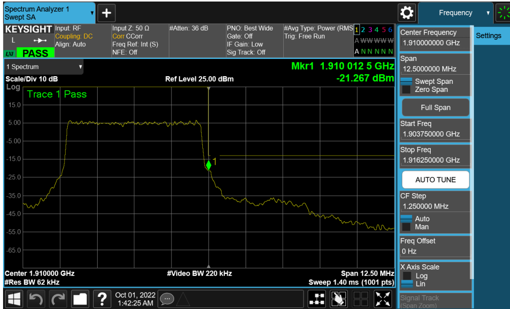
Plot 7-270. Upper Band Edge Plot (NR Band n2 – 5MHz QPSK – Full RB - Ant F)
