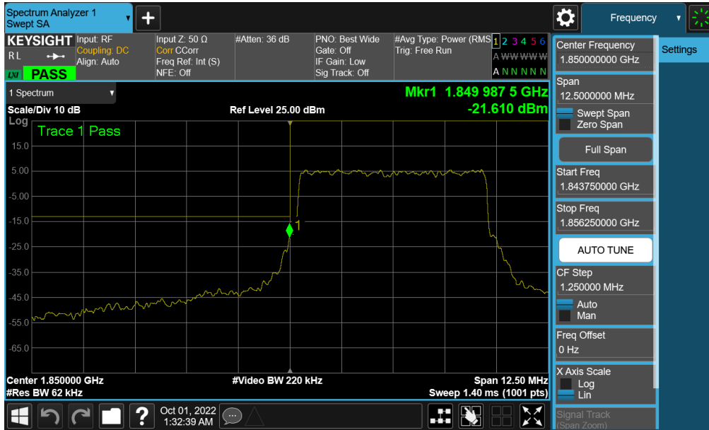
Plot 7-268. Lower Band Edge Plot (NR Band n25/2 – 5MHz QPSK – Full RB - Ant F)
