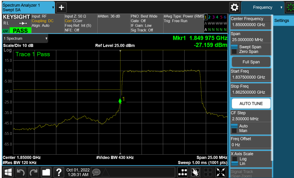
Plot 7-262. Lower Band Edge Plot (NR Band n25/2 - 10MHz QPSK – Full RB - Ant F)
