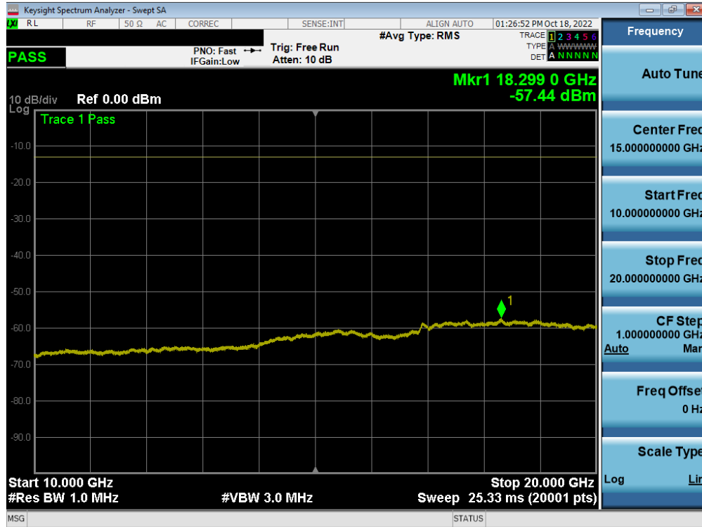
Plot 7-105. Conducted Spurious Plot (WCDMA Ch. 9538)
