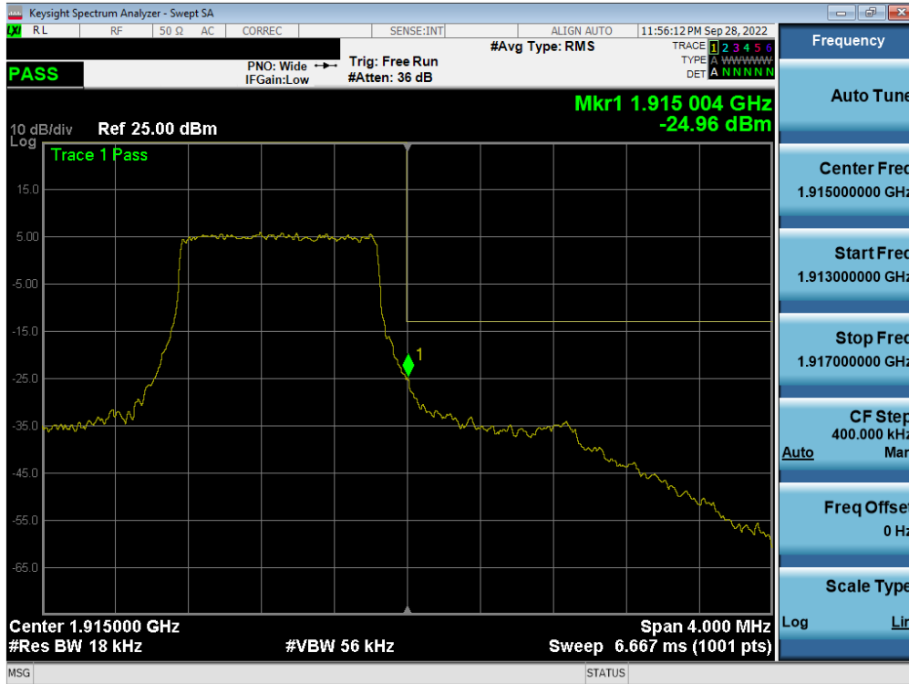
Plot 7-158. Upper Band Edge Plot (LTE Band 25 – 1.4MHz QPSK – Full RB - Ant A)
