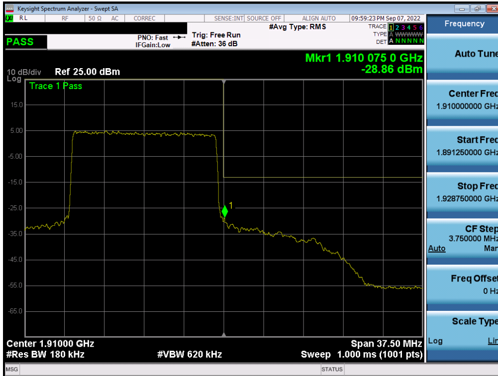
Plot 7-132. Upper Band Edge Plot (LTE Band 2 - 15MHz QPSK – Full RB - Ant A)
