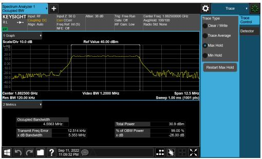
Plot 7-31. Occupied Bandwidth Plot (NR Band n25/2 - 5.0MHz DFT-s-OFDM BPSK - Full RB - Ant A)
