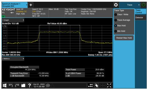
Plot 7-62. Occupied Bandwidth Plot (NR Band n25/2 - 15.0MHz CP-OFDM QPSK - Full RB - Ant F)
