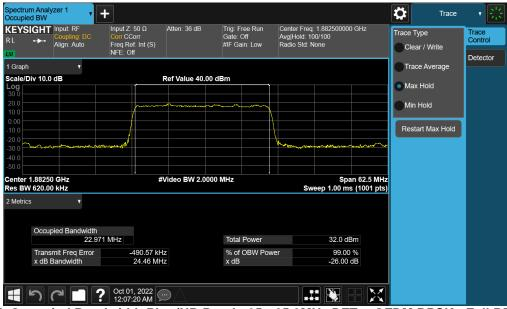
Plot 7-55. Occupied Bandwidth Plot (NR Band n25 - 25.0MHz DFT-s-OFDM BPSK - Full RB - Ant F)
