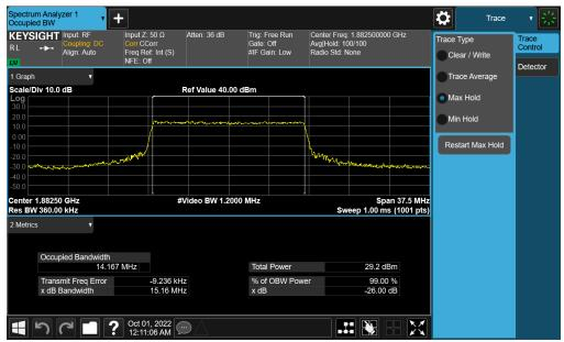
Plot 7-63. Occupied Bandwidth Plot (NR Band n25/2 - 15.0MHz CP-OFDM 16QAM - Full RB - Ant F)
