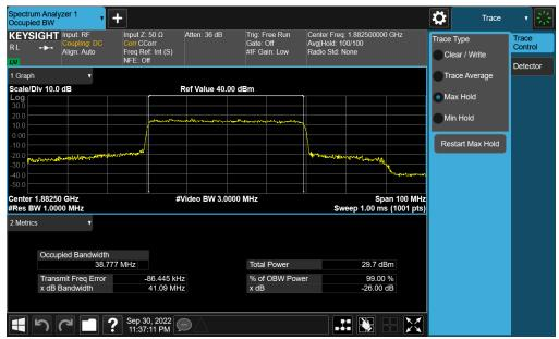
Plot 7-51. Occupied Bandwidth Plot (NR Band n25 - 40.0MHz CP-OFDM 16QAM - Full RB - Ant F)
