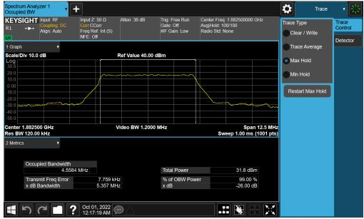
Plot 7-67. Occupied Bandwidth Plot (NR Band n25/2 - 5.0MHz DFT-s-OFDM BPSK - Full RB - Ant F)
