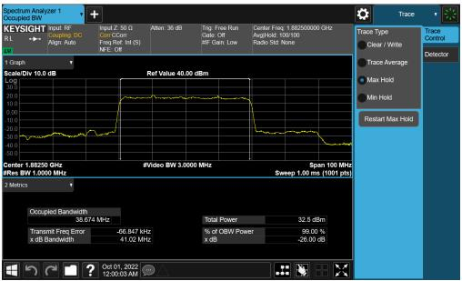
Plot 7-49. Occupied Bandwidth Plot (NR Band n25 - 40.0MHz DFT-s-OFDM BPSK - Full RB - Ant F)
