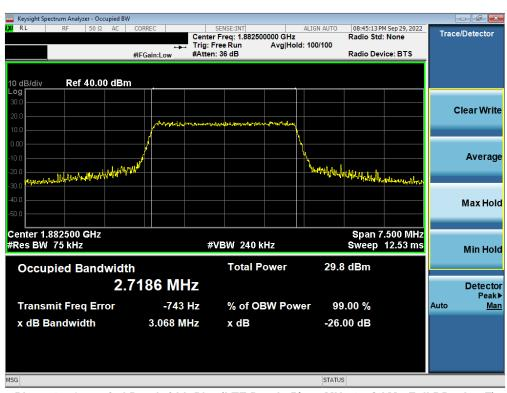
Plot 7-46. Occupied Bandwidth Plot (LTE Band 25/2 - 3MHz 16-QAM - Full RB - Ant F)
