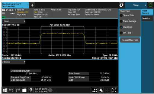
Plot 7-56. Occupied Bandwidth Plot (NR Band n25 - 25.0MHz CP-OFDM QPSK - Full RB - Ant F)
