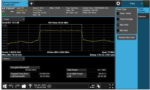
Plot 7-52. Occupied Bandwidth Plot (NR Band n25 - 30.0MHz DFT-s-OFDM BPSK - Full RB - Ant F)
