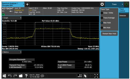
Plot 7-66. Occupied Bandwidth Plot (NR Band n25/2 - 10.0MHz CP-OFDM 16QAM - Full RB - Ant F)
