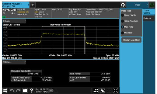
Plot 7-24. Occupied Bandwidth Plot (NR Band n25/2 - 20.0MHz CP-OFDM 16QAM - Full RB - Ant A)
