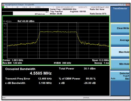
Plot 7-8. Occupied Bandwidth Plot (LTE Band 25/2 - 5MHz 16-QAM - Full RB - Ant A)
