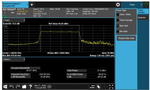
Plot 7-22. Occupied Bandwidth Plot (NR Band n25/2 - 20.0MHz DFT-s-OFDM BPSK - Full RB - Ant A)
