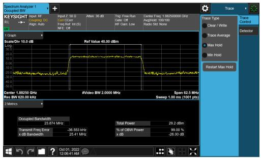
Plot 7-57. Occupied Bandwidth Plot (NR Band n25 - 25.0MHz CP-OFDM 16QAM - Full RB - Ant F)
