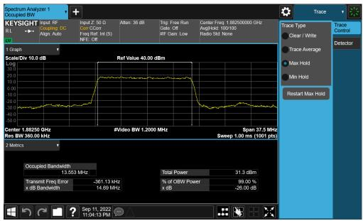
Plot 7-25. Occupied Bandwidth Plot (NR Band n25/2 - 15.0MHz DFT-s-OFDM BPSK - Full RB - Ant A)
