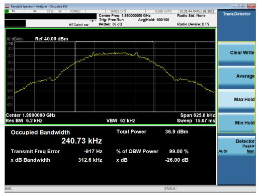
Plot 7-34. Occupied Bandwidth Plot (GPRS, Ch. 661)
