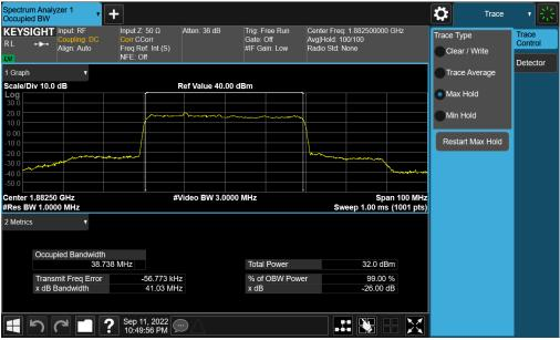
Plot 7-13. Occupied Bandwidth Plot (NR Band n25 - 40.0MHz DFT-s-OFDM BPSK - Full RB - Ant A)
