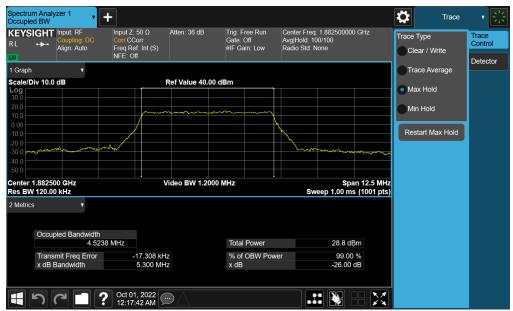
Plot 7-68. Occupied Bandwidth Plot (NR Band n25/2 - 5.0MHz CP-OFDM QPSK - Full RB - Ant F)
