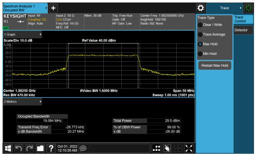
Plot 7-60. Occupied Bandwidth Plot (NR Band n25/2 - 20.0MHz CP-OFDM 16QAM - Full RB - Ant F)
