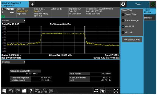
Plot 7-27. Occupied Bandwidth Plot (NR Band n25/2 - 15.0MHz CP-OFDM 16QAM - Full RB - Ant A)
