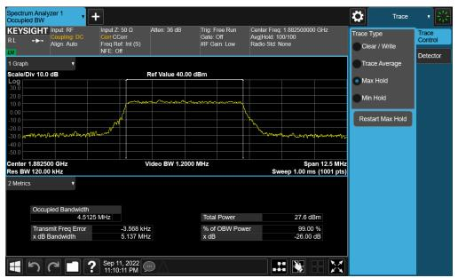
Plot 7-33. Occupied Bandwidth Plot (NR Band n25/2 - 5.0MHz CP-OFDM 16QAM - Full RB - Ant A)
