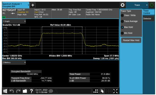
Plot 7-61. Occupied Bandwidth Plot (NR Band n25/2 - 15.0MHz DFT-s-OFDM BPSK - Full RB - Ant F)
