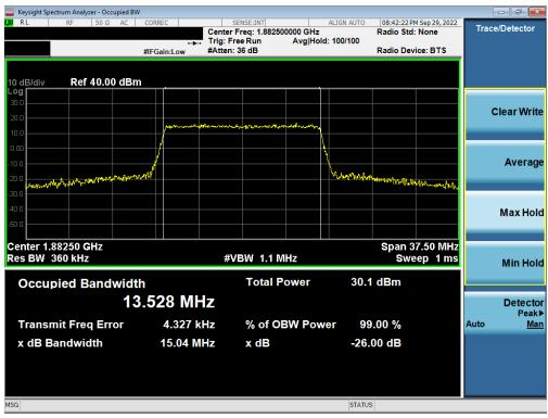
Plot 7-40. Occupied Bandwidth Plot (LTE Band 25/2 - 15MHz 16-QAM - Full RB - Ant F)
