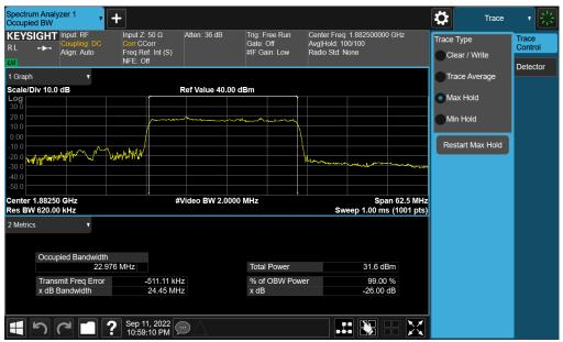
Plot 7-19. Occupied Bandwidth Plot (NR Band n25 - 25.0MHz DFT-s-OFDM BPSK - Full RB - Ant A)
