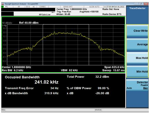
Plot 7-35. Occupied Bandwidth Plot (EDGE, Ch. 661)
