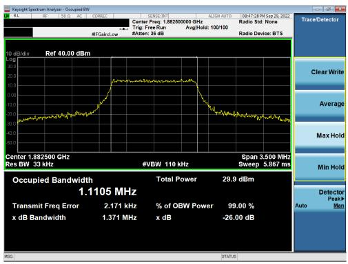
Plot 7-48. Occupied Bandwidth Plot (LTE Band 25/2 - 1.4MHz 16-QAM - Full RB - Ant F)
