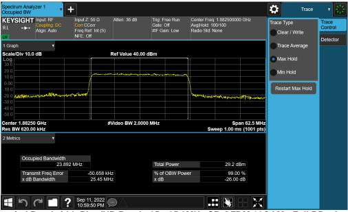
Plot 7-21. Occupied Bandwidth Plot (NR Band n25 - 25.0MHz CP-OFDM 16QAM - Full RB - Ant A)
