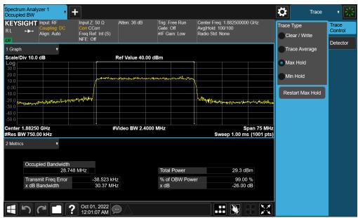
Plot 7-54. Occupied Bandwidth Plot (NR Band n25 - 30.0MHz CP-OFDM 16QAM - Full RB - Ant F)
