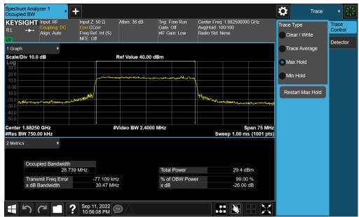
Plot 7-18. Occupied Bandwidth Plot (NR Band n25 - 30.0MHz CP-OFDM 16QAM - Full RB - Ant A)
