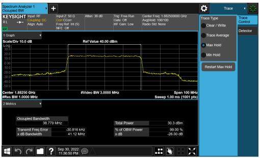
Plot 7-50. Occupied Bandwidth Plot (NR Band n25 - 40.0MHz CP-OFDM QPSK - Full RB - Ant F)
