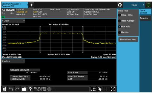
Plot 7-53. Occupied Bandwidth Plot (NR Band n25 - 30.0MHz CP-OFDM QPSK - Full RB - Ant F)
