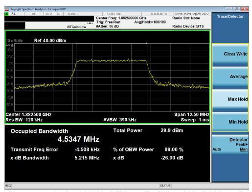
Plot 7-44. Occupied Bandwidth Plot (LTE Band 25/2 - 5MHz 16-QAM - Full RB - Ant F)
