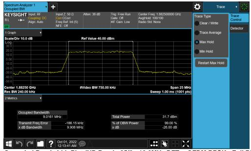
Plot 7-64. Occupied Bandwidth Plot (NR Band n25/2 - 10.0MHz DFT-s-OFDM BPSK - Full RB - Ant F)
