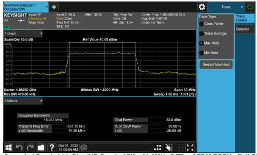
Plot 7-58. Occupied Bandwidth Plot (NR Band n25/2 - 20.0MHz DFT-s-OFDM BPSK - Full RB - Ant F)
