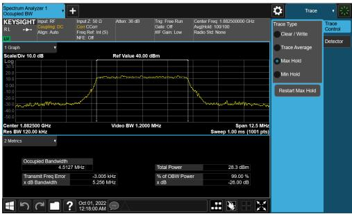
Plot 7-69. Occupied Bandwidth Plot (NR Band n25/2 - 5.0MHz CP-OFDM 16QAM - Full RB - Ant F)
