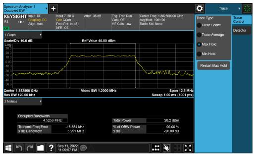
Plot 7-32. Occupied Bandwidth Plot (NR Band n25/2 - 5.0MHz CP-OFDM QPSK - Full RB - Ant A)
