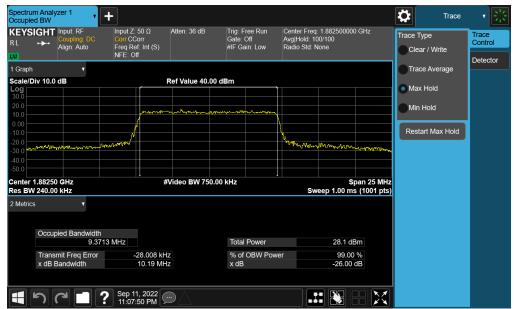
Plot 7-30. Occupied Bandwidth Plot (NR Band n25/2 - 10.0MHz CP-OFDM 16QAM - Full RB - Ant A)
