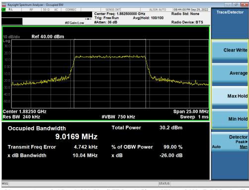
Plot 7-42. Occupied Bandwidth Plot (LTE Band 25/2 - 10MHz 16-QAM - Full RB - Ant F)
