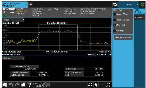
Plot 7-28. Occupied Bandwidth Plot (NR Band n25/2 - 10.0MHz DFT-s-OFDM BPSK - Full RB - Ant A)
