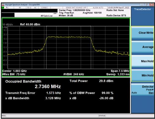
Plot 7-10. Occupied Bandwidth Plot (LTE Band 25/2 - 3MHz 16-QAM - Full RB - Ant A)
