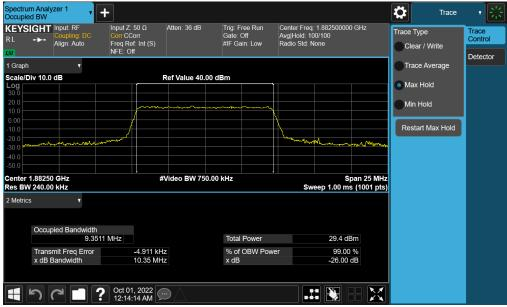
Plot 7-65. Occupied Bandwidth Plot (NR Band n25/2 - 10.0MHz CP-OFDM QPSK - Full RB - Ant F)
