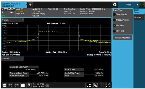
Plot 7-23. Occupied Bandwidth Plot (NR Band n25/2 - 20.0MHz CP-OFDM QPSK - Full RB - Ant A)
