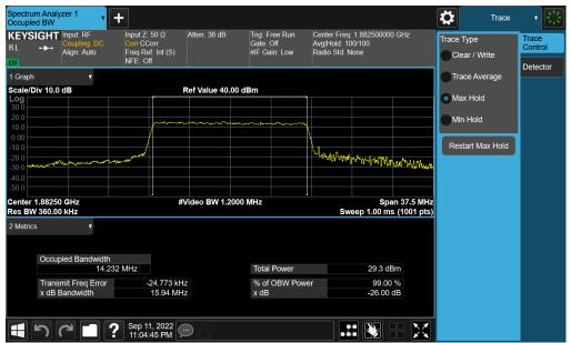
Plot 7-26. Occupied Bandwidth Plot (NR Band n25/2 - 15.0MHz CP-OFDM QPSK - Full RB - Ant A)
