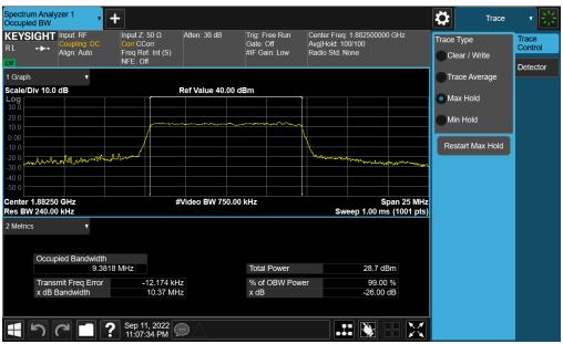
Plot 7-29. Occupied Bandwidth Plot (NR Band n25/2 - 10.0MHz CP-OFDM QPSK - Full RB - Ant A)
