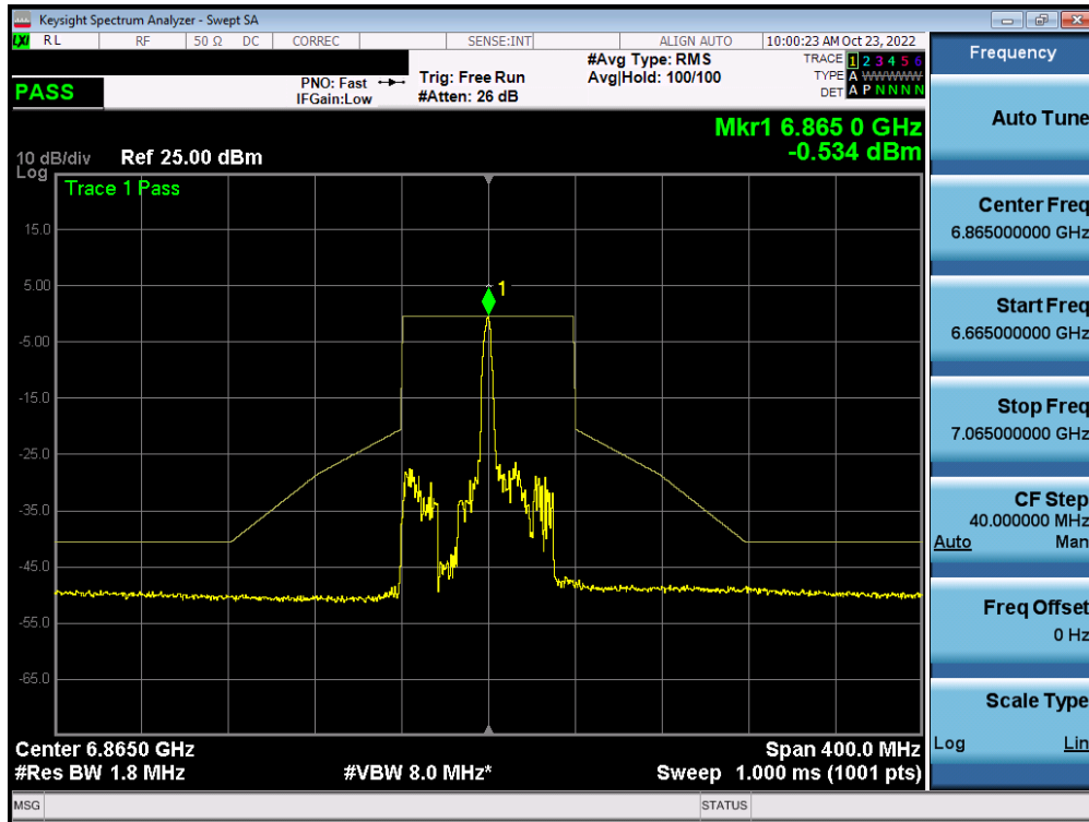
Plot 7-574. In-Band Emission Plot MIMO ANT2 (80MHz BW 802.11ax (26 Tones) (UNII Band 7) – Ch. 183) – LPI
