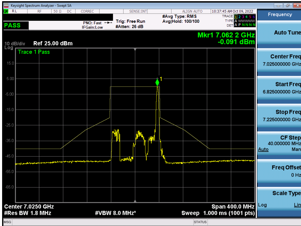
Plot 7-475. In-Band Emission Plot MIMO ANT1 (80MHz BW 802.11ax (26 Tones) (UNII Band 8) – Ch. 215) – LPI
