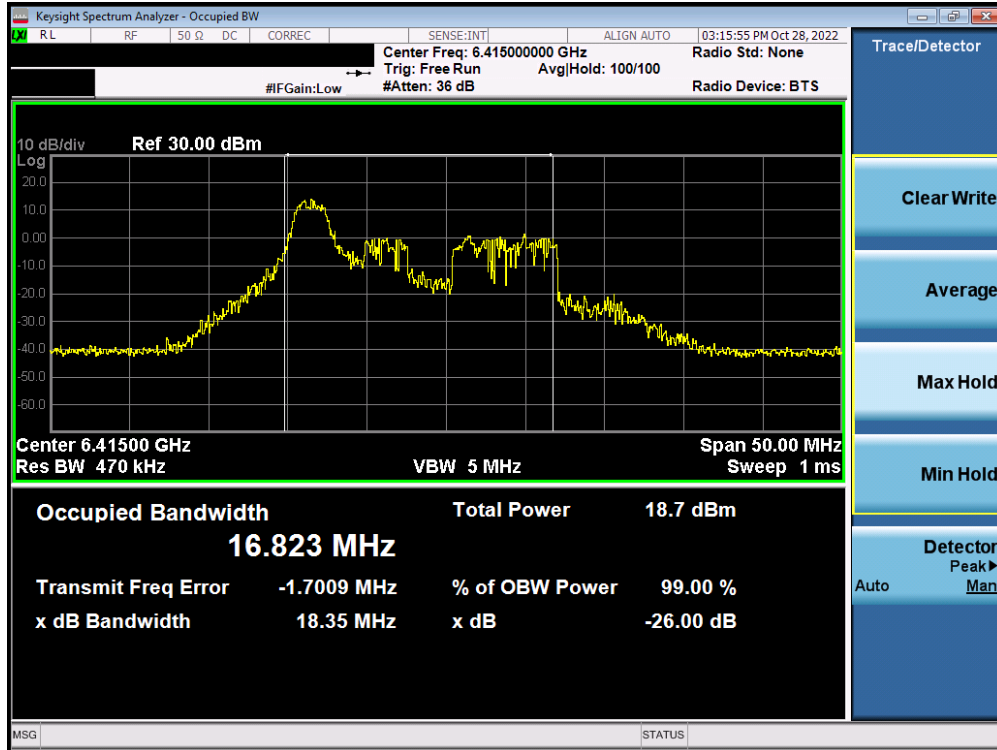
Plot 7-152. Occupied Bandwidth Plot MIMO ANT2 (20MHz BW 802.11ax (26 Tones) UNII Band 5) – Ch. 93) - SP
