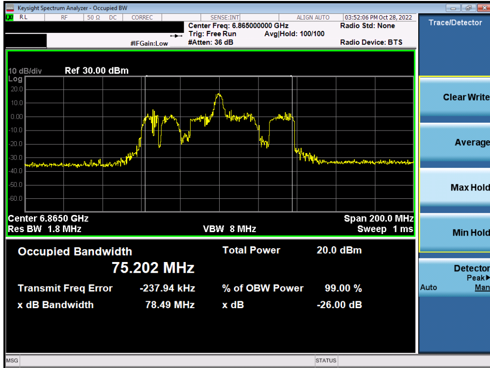
Plot 7-170. Occupied Bandwidth Plot MIMO ANT2 (80MHz BW 802.11ax (26 Tones) (UNII Band 7) – Ch. 183) – SP
