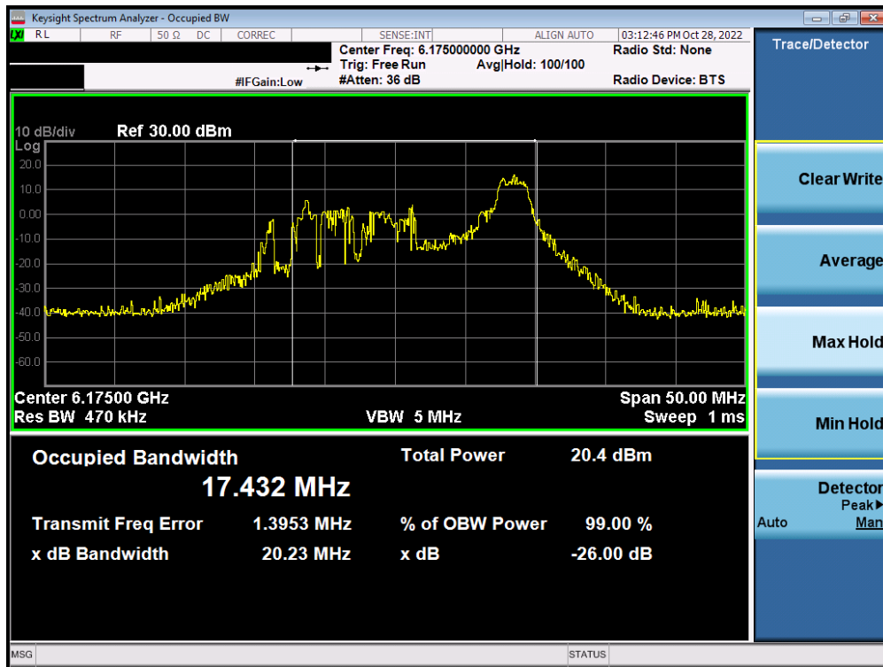
Plot 7-151. Occupied Bandwidth Plot MIMO ANT2 (20MHz BW 802.11ax (26 Tones) (UNII Band 5) – Ch. 45) - SP
