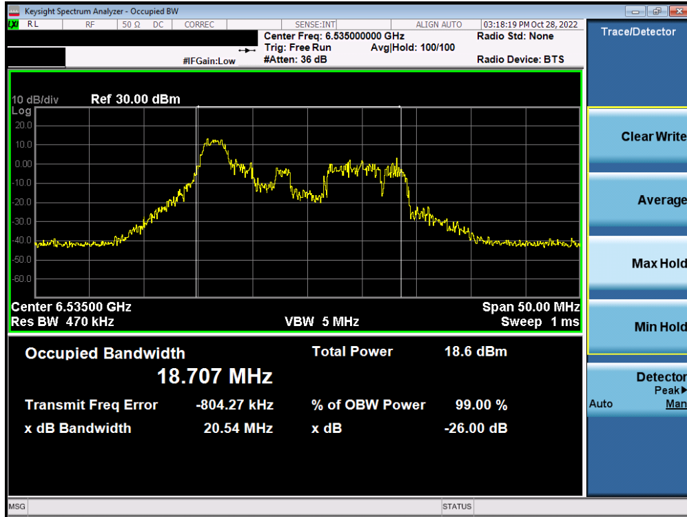
Plot 7-162. Occupied Bandwidth Plot MIMO ANT2 (20MHz BW 802.11ax (26 Tones) (UNII Band 7) – Ch. 117) – SP
