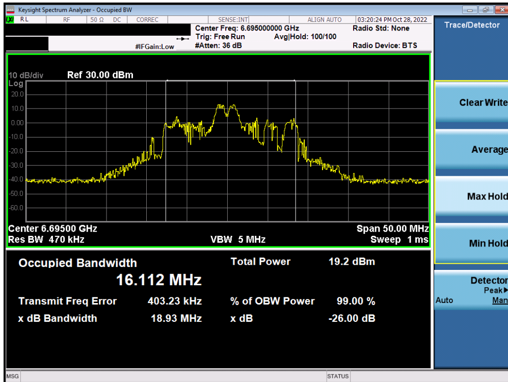
Plot 7-163. Occupied Bandwidth Plot MIMO ANT2 (20MHz BW 802.11ax (26 Tones) (UNII Band 7) – Ch. 149) – SP
