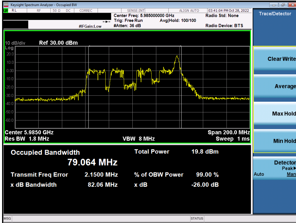
Plot 7-156. Occupied Bandwidth Plot MIMO ANT2 (80MHz BW 802.11ax (26 Tones) (UNII Band 5) – Ch. 7) - SP
