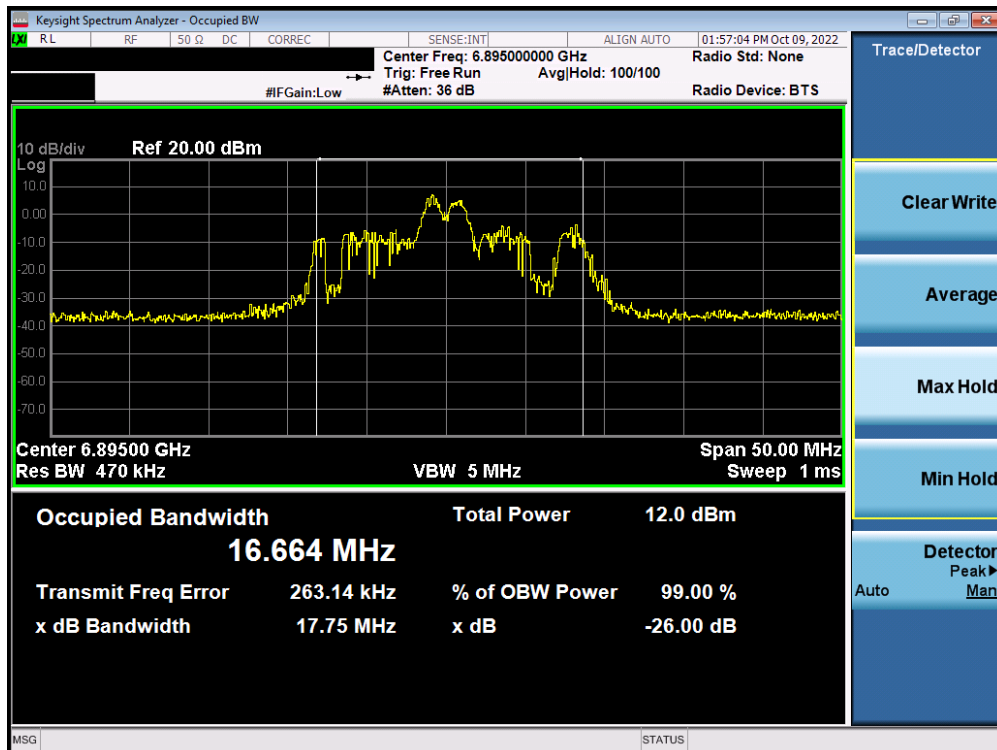
Plot 7-141. Occupied Bandwidth Plot MIMO ANT2 (20MHz BW 802.11ax (26 Tones) (UNII Band 8) – Ch. 189) – LPI
