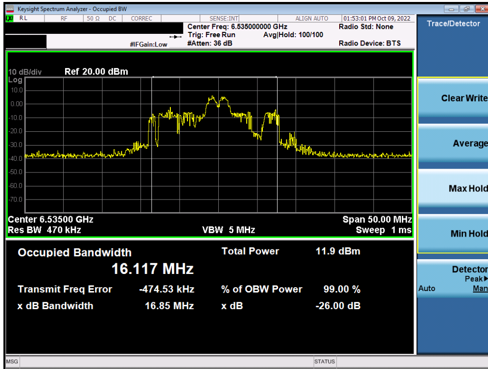
Plot 7-130. Occupied Bandwidth Plot MIMO ANT2 (20MHz BW 802.11ax (26 Tones) (UNII Band 7) – Ch. 117) – LPI
