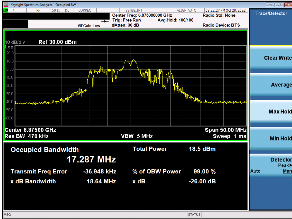
Plot 7-164. Occupied Bandwidth Plot MIMO ANT2 (20MHz BW 802.11ax (26 Tones) (UNII Band 7) – Ch. 185) – SP
