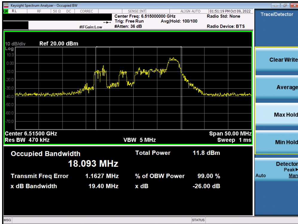
Plot 7-124. Occupied Bandwidth Plot MIMO ANT2 (20MHz BW 802.11ax (26 Tones) (UNII Band 6) – Ch. 113) – LPI
