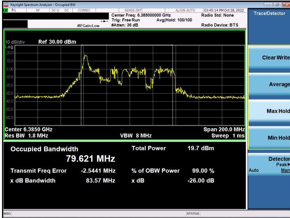
Plot 7-158. Occupied Bandwidth Plot MIMO ANT2 (80MHz BW 802.11ax (26 Tones) (UNII Band 5) – Ch. 87) - SP
