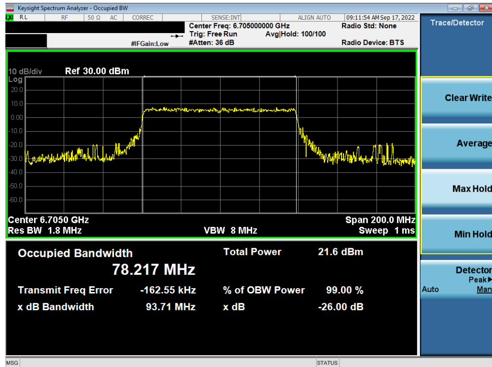
Plot 7-97. Occupied Bandwidth Plot MIMO ANT1 (80MHz BW 802.11ax (Full Tone) (UNII Band 7) – Ch. 151) – LPI/SP
