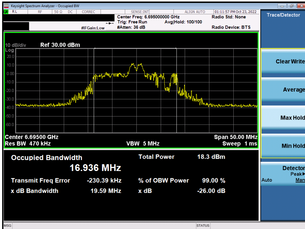
Plot 7-54. Occupied Bandwidth Plot MIMO ANT1 (20MHz BW 802.11ax (26 Tones) (UNII Band 7) – Ch. 149) – SP
