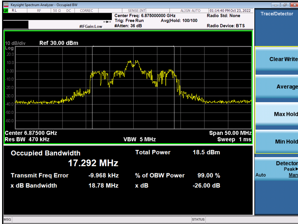
Plot 7-55. Occupied Bandwidth Plot MIMO ANT1 (20MHz BW 802.11ax (26 Tones) (UNII Band 7) – Ch. 185) – SP
