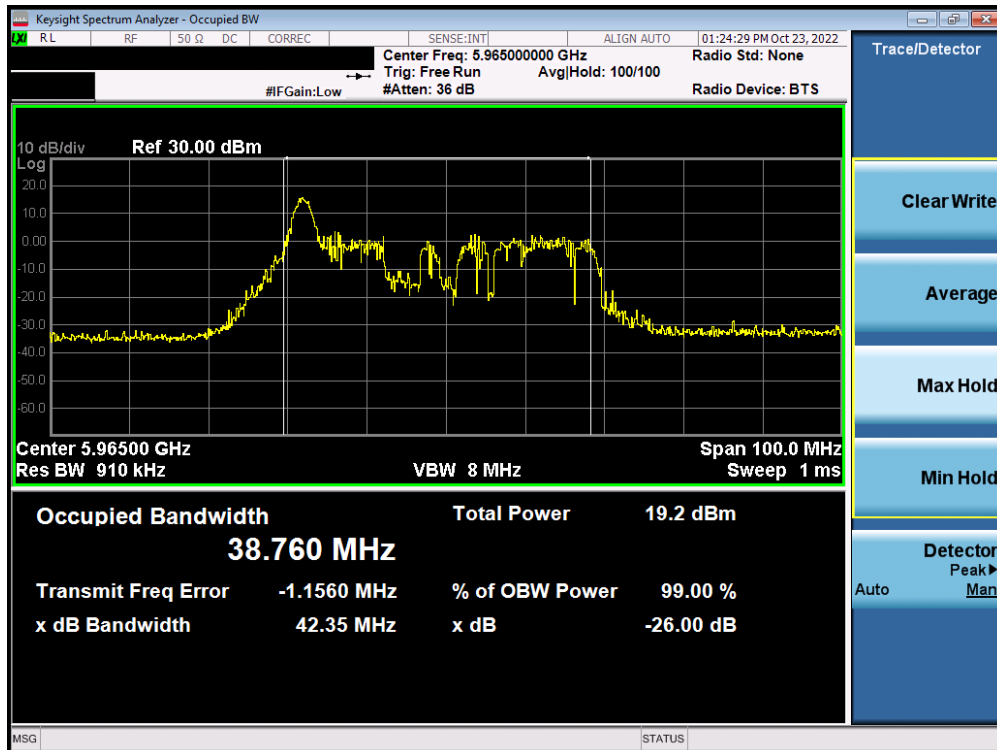
Plot 7-44. Occupied Bandwidth Plot MIMO ANT1 (40MHz BW 802.11ax (26 Tones) (UNII Band 5) – Ch. 3) - SP
