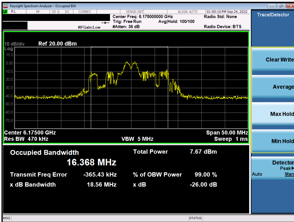
Plot 7-111. Occupied Bandwidth Plot MIMO ANT2 (20MHz BW 802.11ax (26 Tones) (UNII Band 5) – Ch. 45) – LPI
