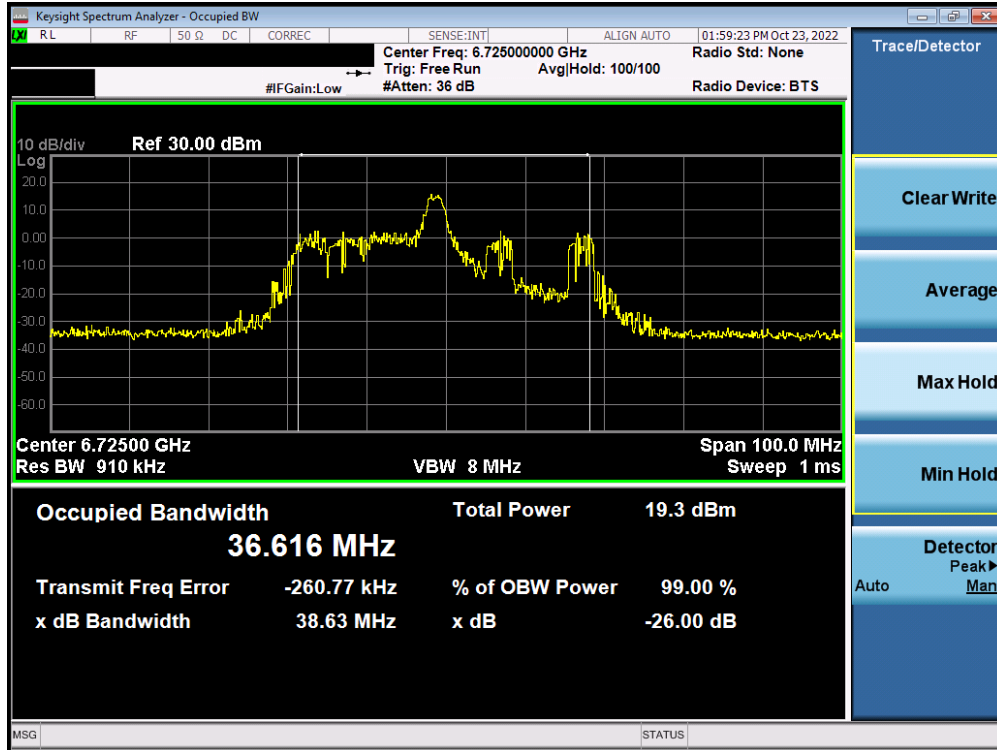
Plot 7-57. Occupied Bandwidth Plot MIMO ANT1 (40MHz BW 802.11ax (26 Tones) (UNII Band 7) – Ch. 155) – SP
