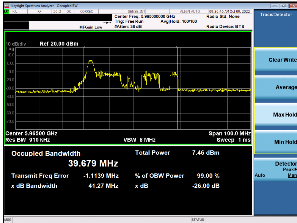
Plot 7-4. Occupied Bandwidth Plot MIMO ANT1 (40MHz BW 802.11ax (26 Tones) (UNII Band 5) – Ch. 3) – LPI
