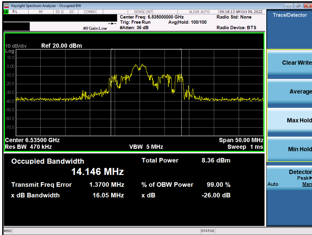
Plot 7-21. Occupied Bandwidth Plot MIMO ANT1 (20MHz BW 802.11ax (26 Tones) (UNII Band 7) – Ch. 117) – LPI
