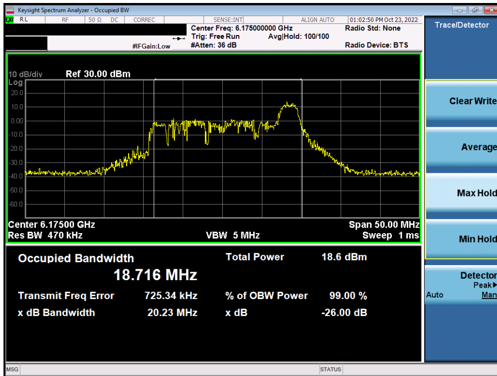
Plot 7-42. Occupied Bandwidth Plot MIMO ANT1 (20MHz BW 802.11ax (26 Tones) (UNII Band 5) – Ch. 45) - SP
