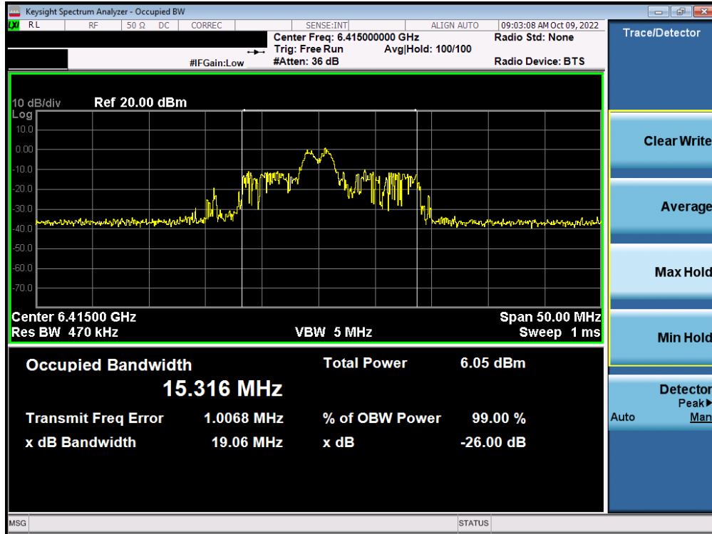
Plot 7-3. Occupied Bandwidth Plot MIMO ANT1 (20MHz BW 802.11ax (26 Tones) UNII Band 5) – Ch. 93) – LPI
