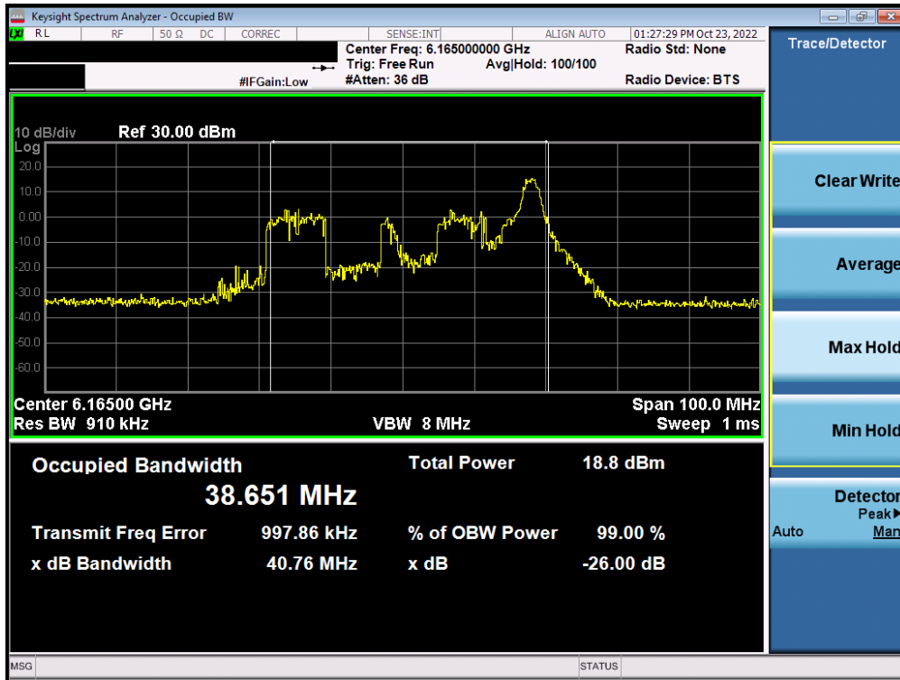
Plot 7-45. Occupied Bandwidth Plot MIMO ANT1 (40MHz BW 802.11ax (26 Tones) (UNII Band 5) – Ch. 43) - SP
