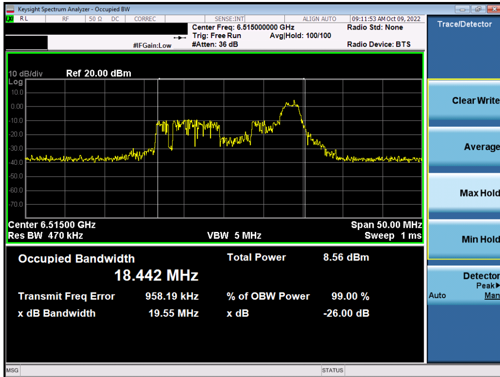
Plot 7-15. Occupied Bandwidth Plot MIMO ANT1 (20MHz BW 802.11ax (26 Tones) (UNII Band 6) – Ch. 113) – LPI
