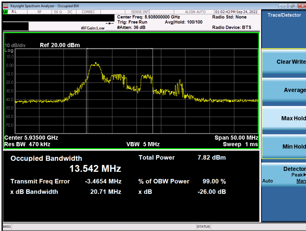
Plot 7-110. Occupied Bandwidth Plot MIMO ANT2 (20MHz BW 802.11ax (26 Tones) UNII Band 5) – Ch. 2 – LPI
