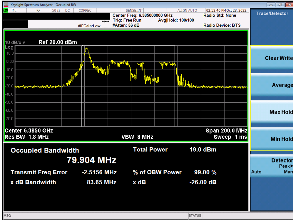
Plot 7-49. Occupied Bandwidth Plot MIMO ANT1 (80MHz BW 802.11ax (26 Tones) (UNII Band 5) – Ch. 87) - SP
