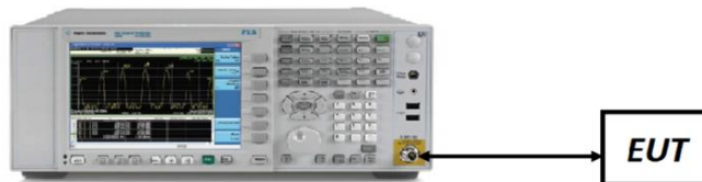
Figure 7-2. Test Instrument & Measurement Setup
