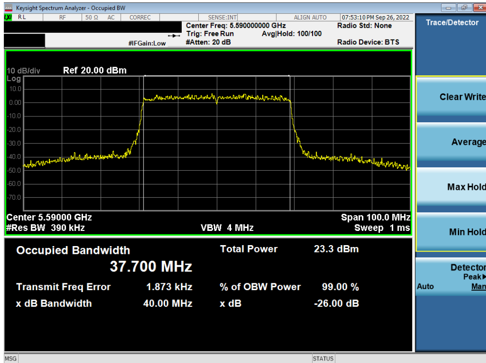
Plot 7-46. 26dB Bandwidth Plot ANT1 (40MHz BW 802.11ax (UNII Band 2C) – Ch. 118)
