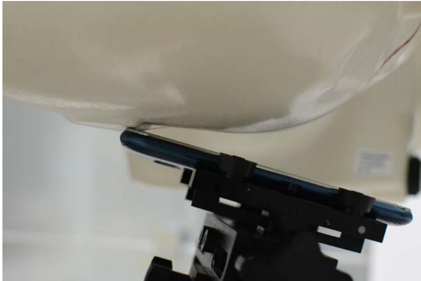
SAR Test Setup Photo 2: Right Tilt
