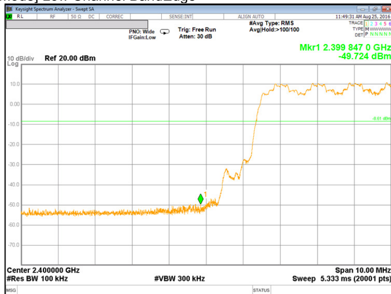
[8PSK Hopping Mode] High Channel BandEdge
