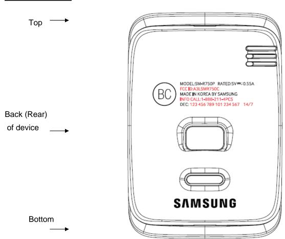
FCC ID is printed on bottom of the device
