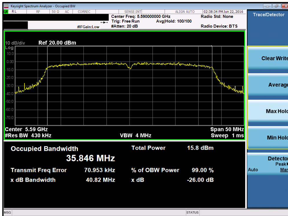
Plot 7-26. 26dB Bandwidth Plot (40MHz BW 802.11n (UNII Band 2C) – Ch. 118)
