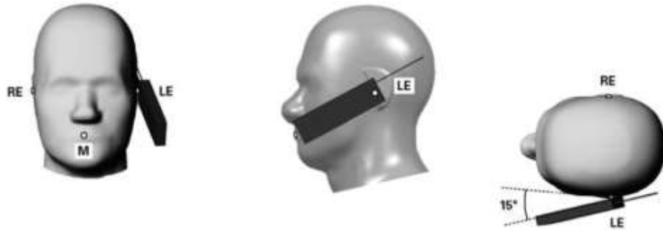
Figure 8.5. Tilt 15° position of the wireless device
