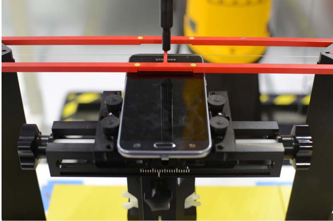
Figure 18-1 Ear Reference Point HAC Phantom Alignment
