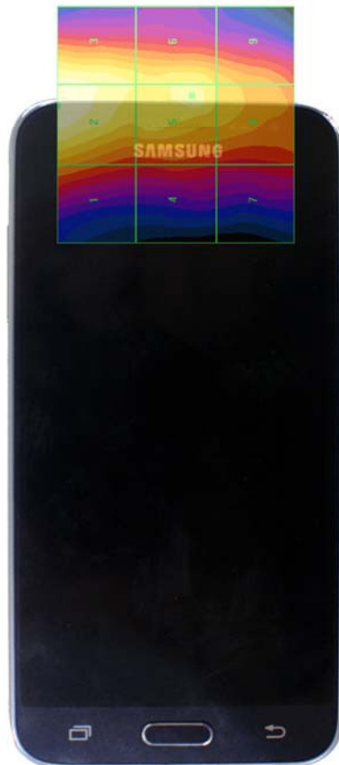
Figure 18-4 E-Field WD Scan overlay
