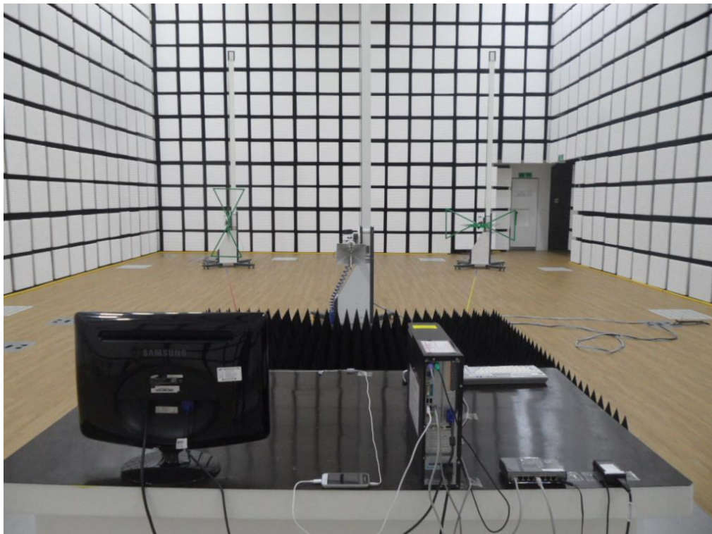
[ Radiated Disturbance for Above 1 GHz – Rear ]
