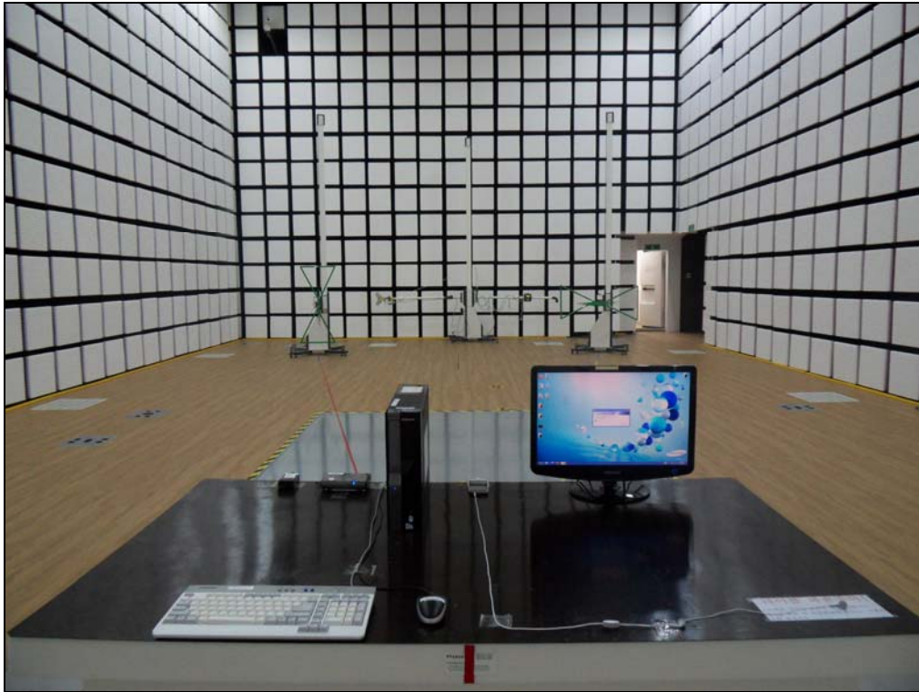
[ Radiated Disturbance for Below 1 GHz – Front ]
