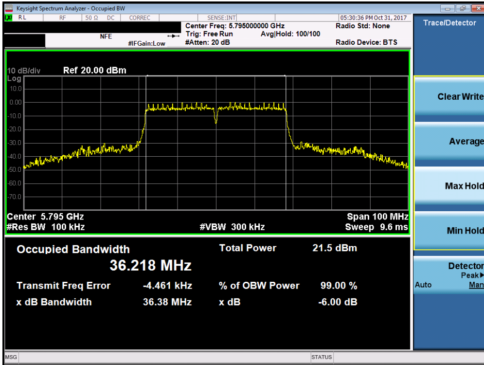
Plot 7-68. 6dB Bandwidth Plot (40MHz BW 802.11n (UNII Band 3) – Ch. 159)
