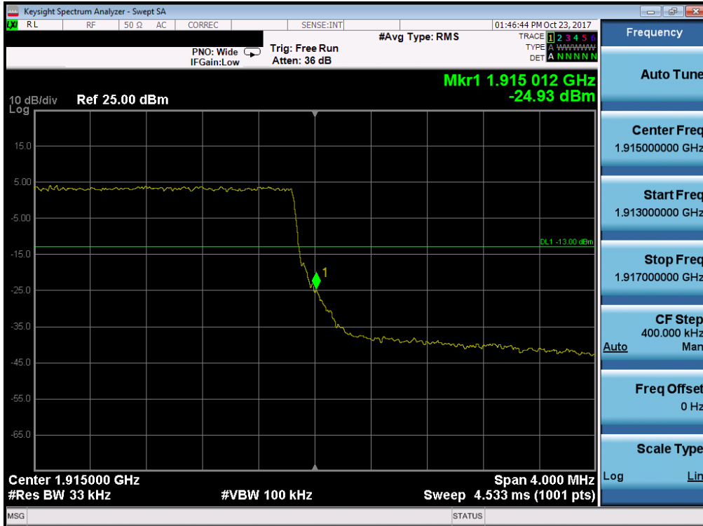
Plot 7-171. Upper Band Edge Plot (Band 25 - 3.0MHz QPSK - Full RB Configuration)
