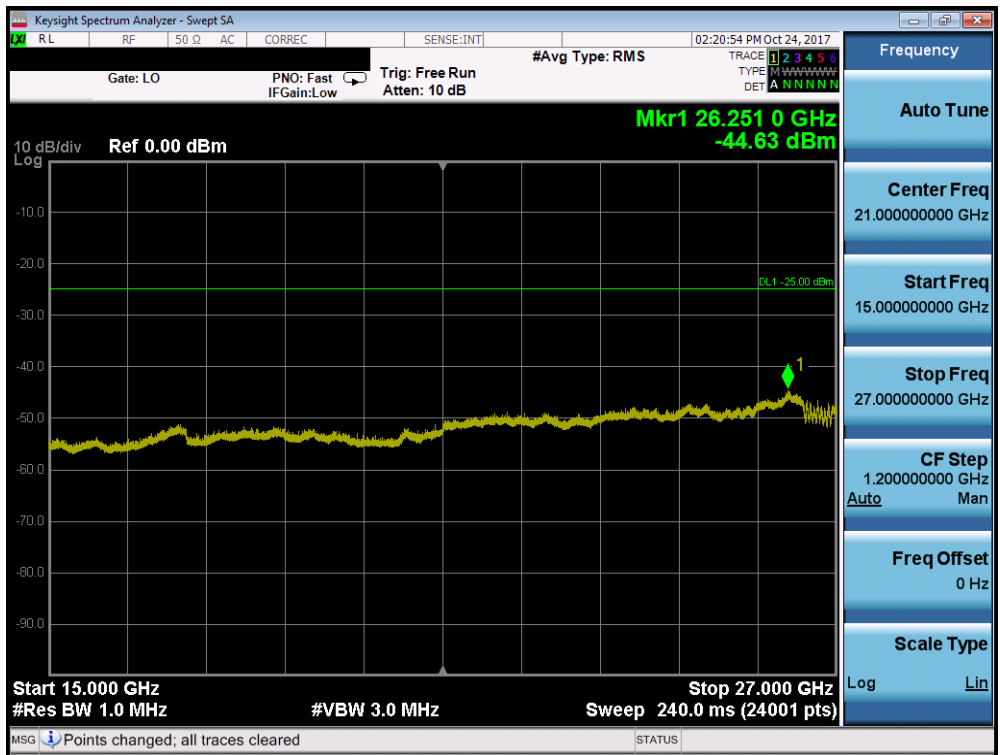
Plot 7-99. Conducted Spurious Plot (Band 41 - 10.0MHz QPSK - RB Size 1, RB Offset 0 - Mid Channel)
