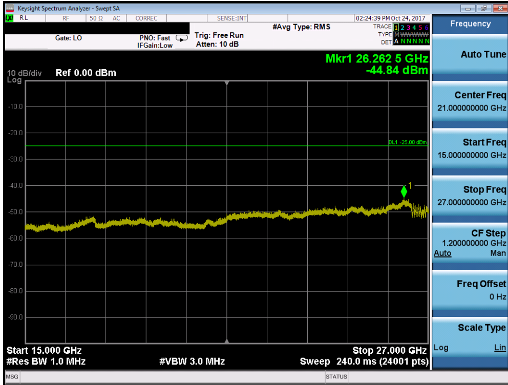
Plot 7-96. Conducted Spurious Plot (Band 41 - 10.0MHz QPSK - RB Size 1, RB Offset 0 - Low Channel)
