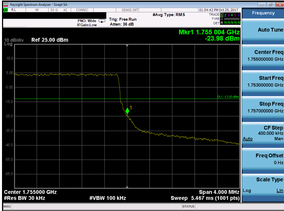
Plot 7-137. Upper Band Edge Plot (Band 4 - 3.0MHz QPSK - Full RB Configuration)
