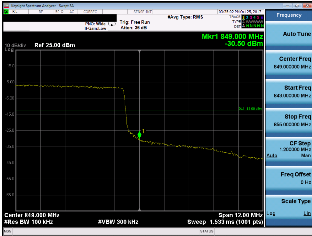
Plot 7-126. Upper Band Edge Plot (Band 26 - 15.0MHz QPSK - Full RB Configuration)
