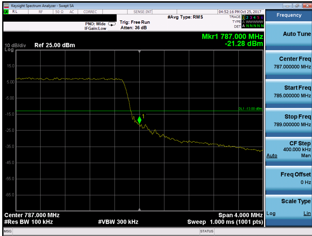
Plot 7-114. Upper Band Edge Plot (Band 13 - 5.0MHz QPSK - Full RB Configuration)
