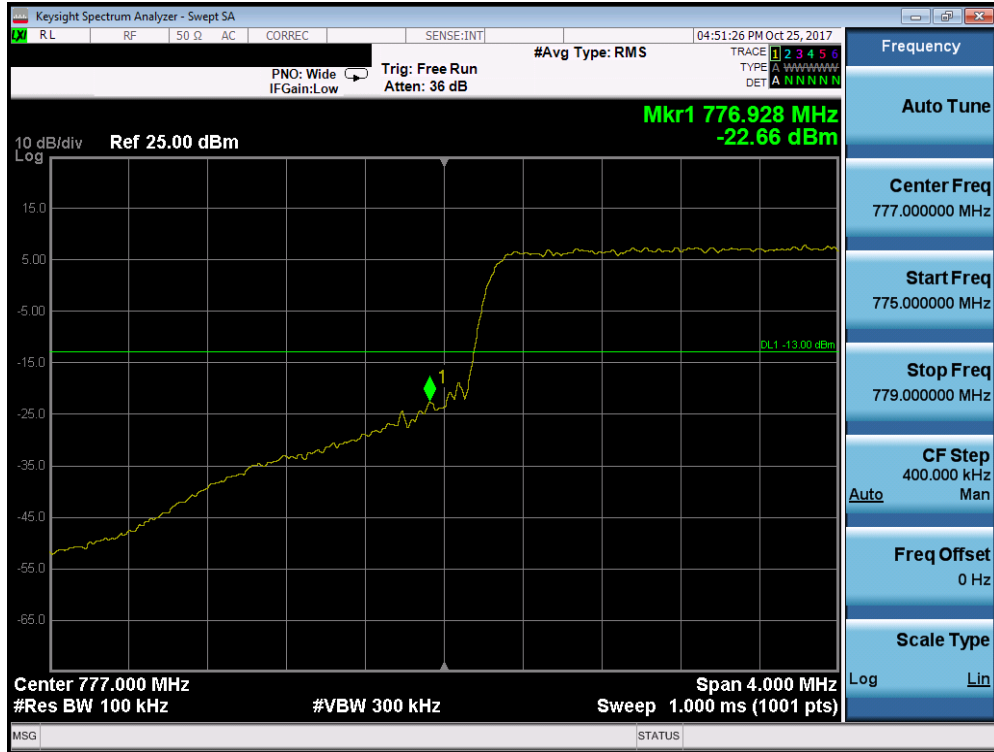
Plot 7-113. Lower Band Edge Plot (Band 13 - 5.0MHz QPSK - Full RB Configuration)
