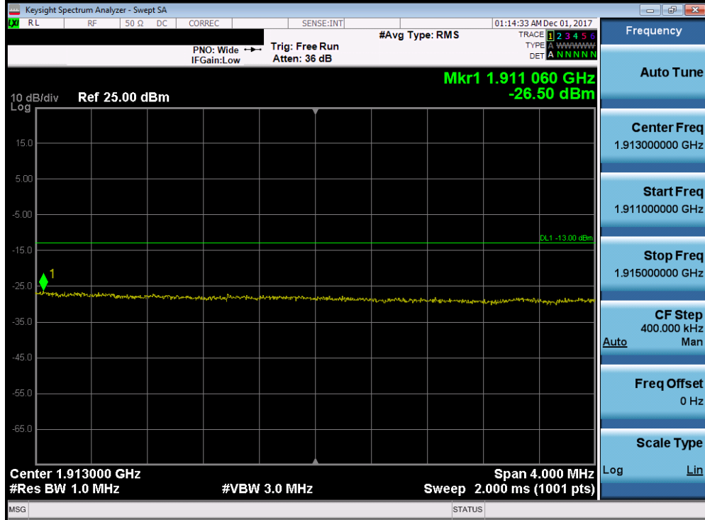
Plot 7-192. Upper Extended Band Edge Plot (Band 2 - 15.0MHz QPSK - Full RB Configuration)
