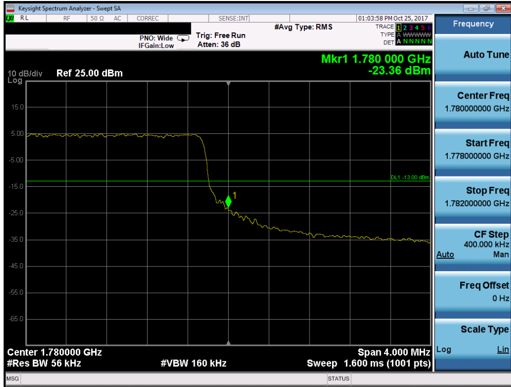
Plot 7-141. Upper Band Edge Plot (Band 66/4 - 5.0MHz QPSK - Full RB Configuration)
