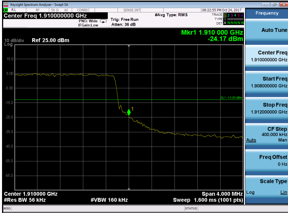
Plot 7-179. Upper Band Edge Plot (Band 2 - 5.0MHz QPSK - Full RB Configuration)
