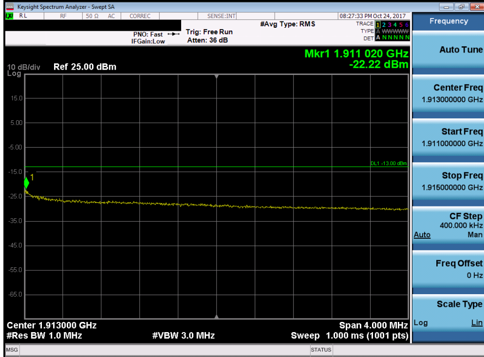
Plot 7-186. Upper Extended Band Edge Plot (Band 2 - 10.0MHz QPSK - Full RB Configuration)
