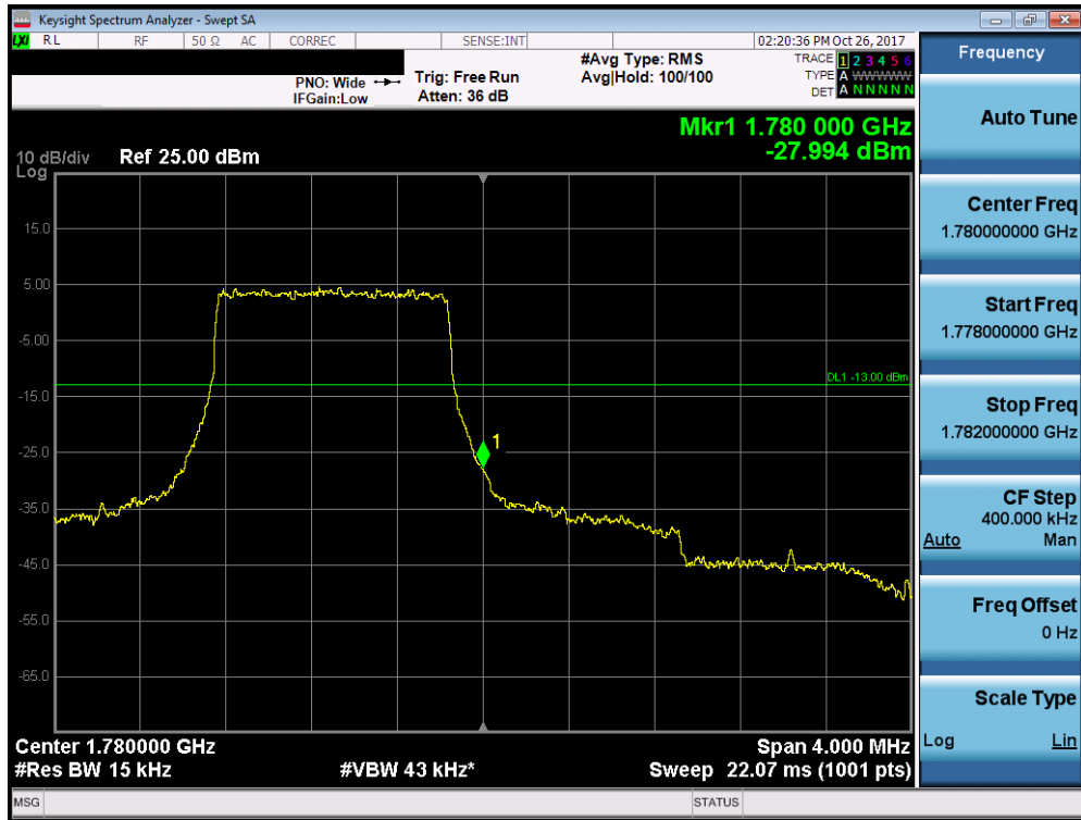
Plot 7-129. Upper Band Edge Plot (Band 66 - 1.4 MHz QPSK - Full RB Configuration)
