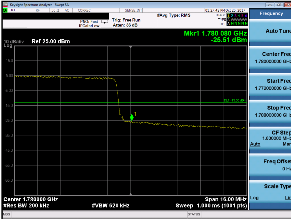
Plot 7-159. Upper Band Edge Plot (Band 66 - 20.0MHz QPSK - Full RB Configuration)
