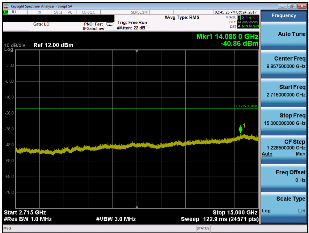
Plot 7-101. Conducted Spurious Plot (Band 41 - 10.0MHz QPSK - RB Size 1, RB Offset 0 - High Channel)
