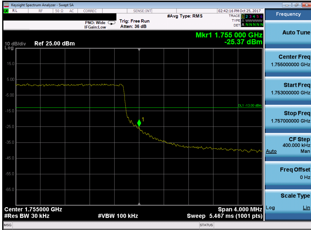
Plot 7-143. Upper Band Edge Plot (Band 4 - 5.0MHz QPSK - Full RB Configuration)
