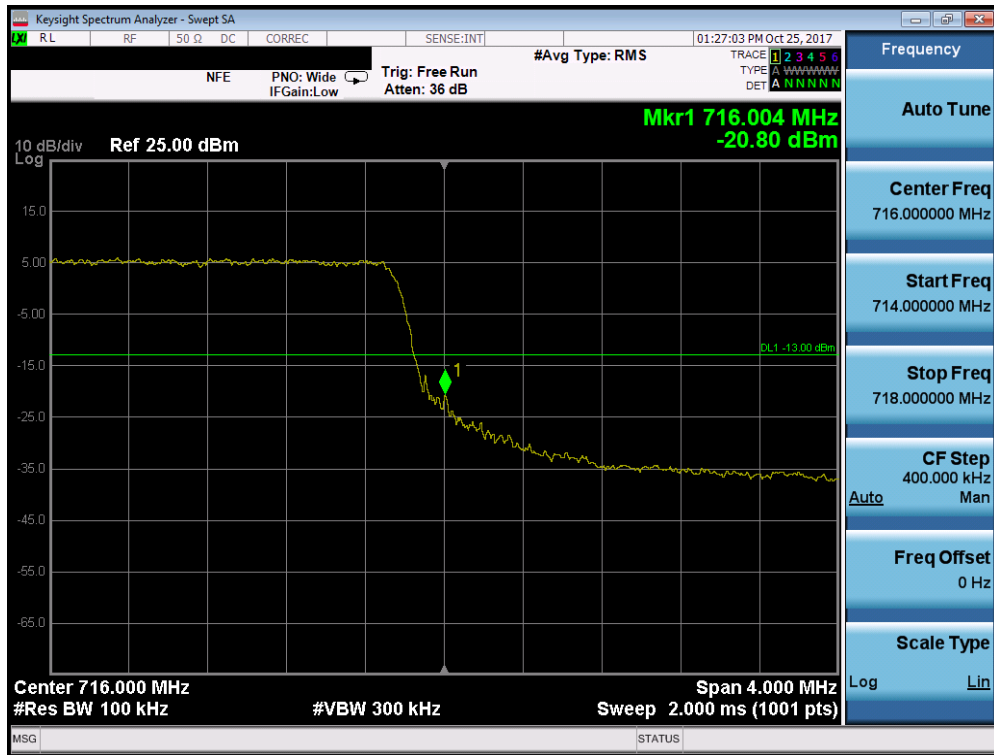
Plot 7-109. Upper Band Edge Plot (Band 12/17 - 5.0MHz QPSK - Full RB Configuration)
