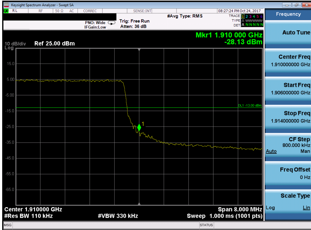
Plot 7-185. Upper Band Edge Plot (Band 2 - 10.0MHz QPSK - Full RB Configuration)
