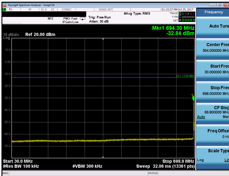
Plot 7-58. Conducted Spurious Plot (Band 12/17 - 10.0MHz QPSK - RB Size 1, RB Offset 0 - Mid Channel)
