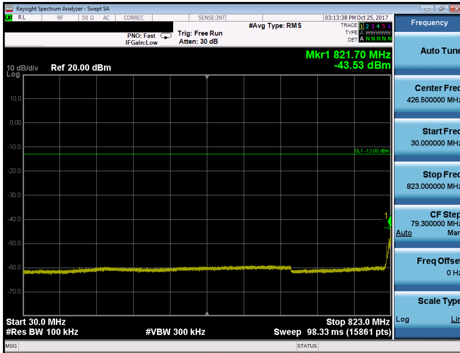
Plot 7-67. Conducted Spurious Plot (Band 26/5 - 3.0MHz QPSK - RB Size 1, RB Offset 0 - Low Channel)
