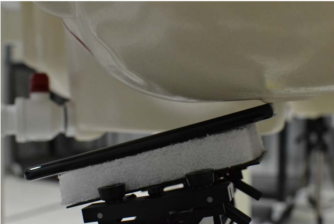
SAR Test Setup Photo 4 – Left Tilt
