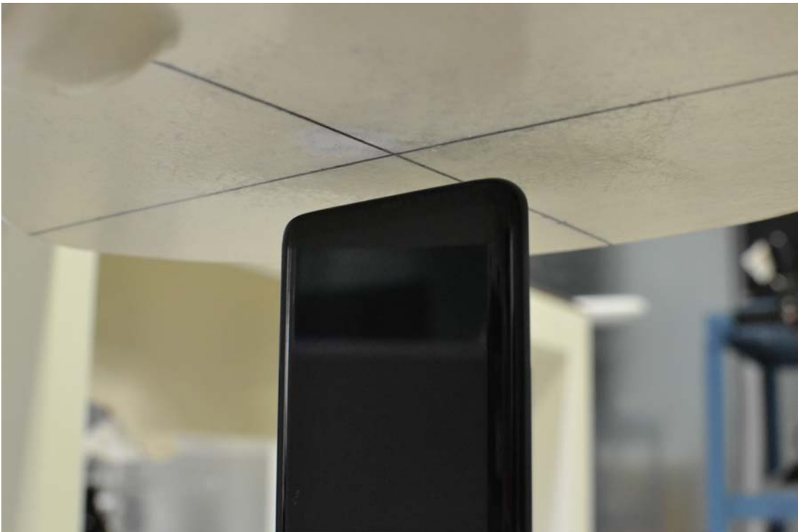
SAR Test Setup Photo 12 – Bottom Edge at 10 mm
