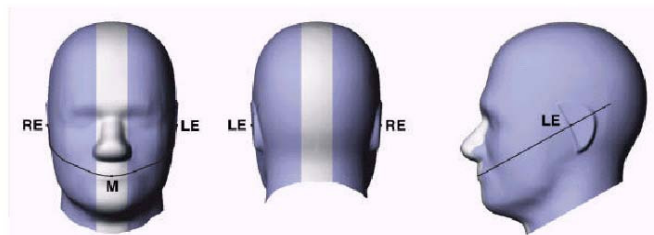
Figure 4-B Front, back and side view of SAM Twin Phantom
