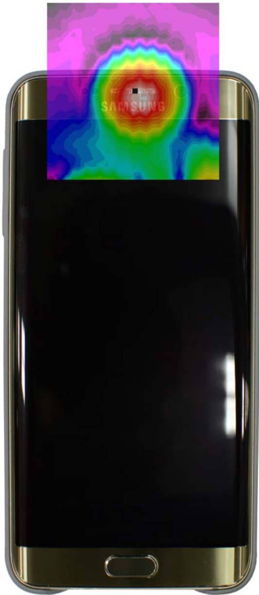
Figure 12-3 Axial T-coil Scan Overlay Magnetic Field Distributions
