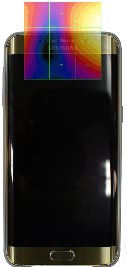
Figure 15-4 E-Field WD Scan overlay
