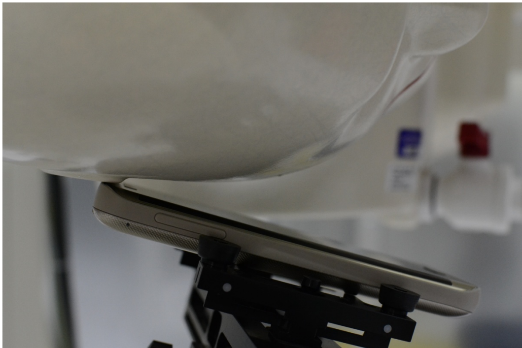
SAR Test Setup Photo 2 - Right Tilt
