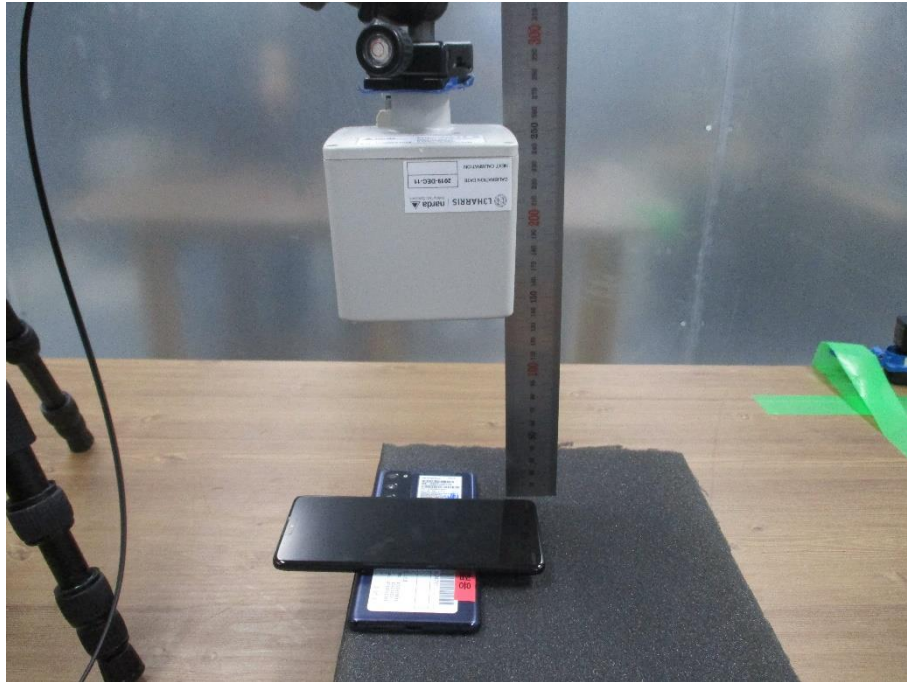
Top charger below client (20cm distance)
