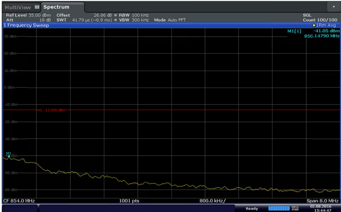
Plot 6-24. Extended Upper Band Edge Plot (Band5 – 1.4MHz – QPSK – RB Size 6)
