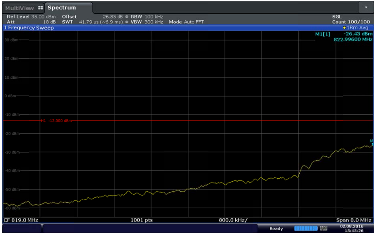
Plot 6-26. Extended Lower Band Edge Plot (Band 5 – 3.0MHz – QPSK – RB Size 15)
