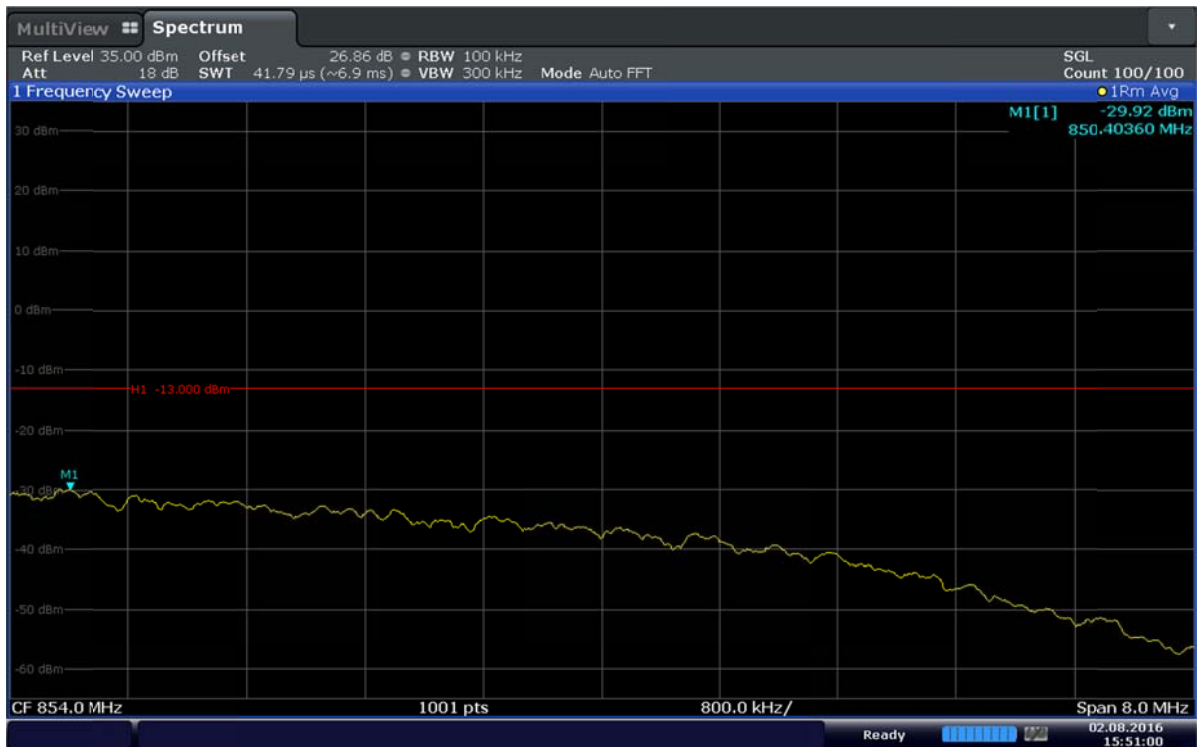
Plot 6-36. Extended Upper Band Edge Plot (Band 5 – 10.0MHz – QPSK – RB Size 50)
