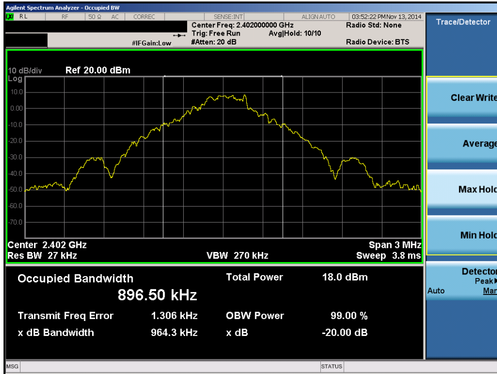
Plot 6-1. 20dB Bandwidth Plot (Bluetooth, 1Mbps – Ch. 0)
