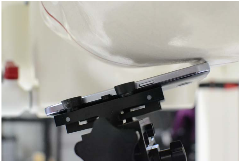
SAR Test Setup Photo 4: Left Tilt
