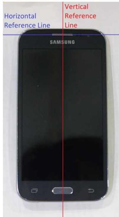
SAR Test Setup Photo 10: Horizontal and Vertical Reference Lines
