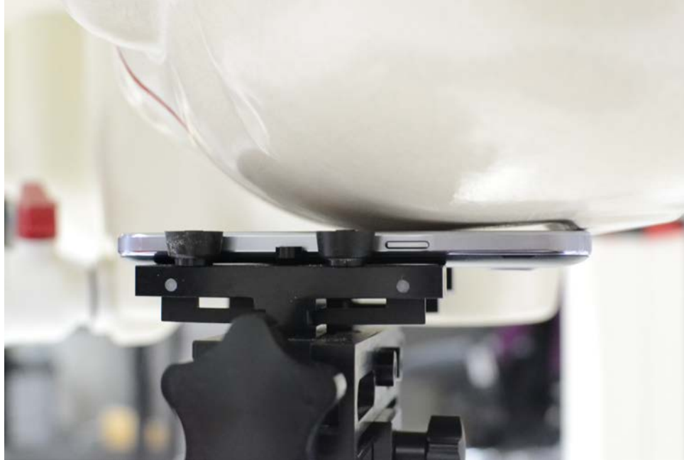
SAR Test Setup Photo 3: Left Cheek
