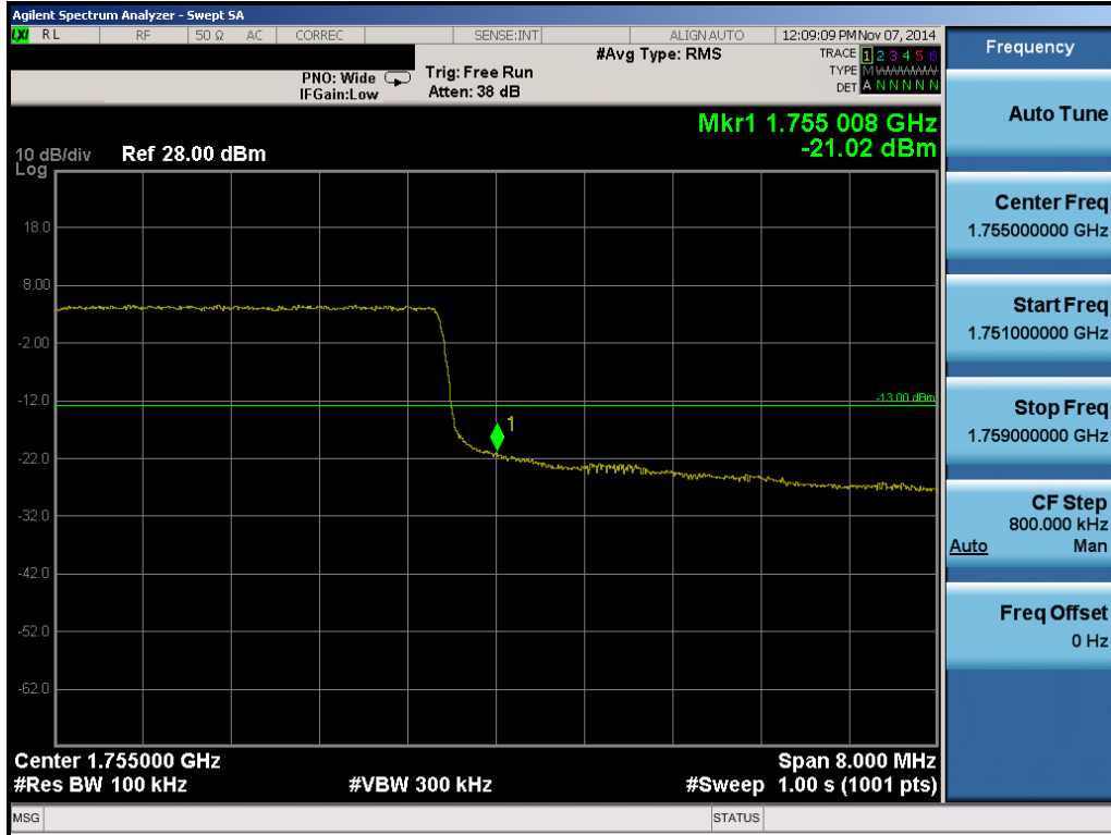
Plot 6-73. Upper Band Edge Plot (Band 4 – 10.0MHz QPSK – RB Size 50)
