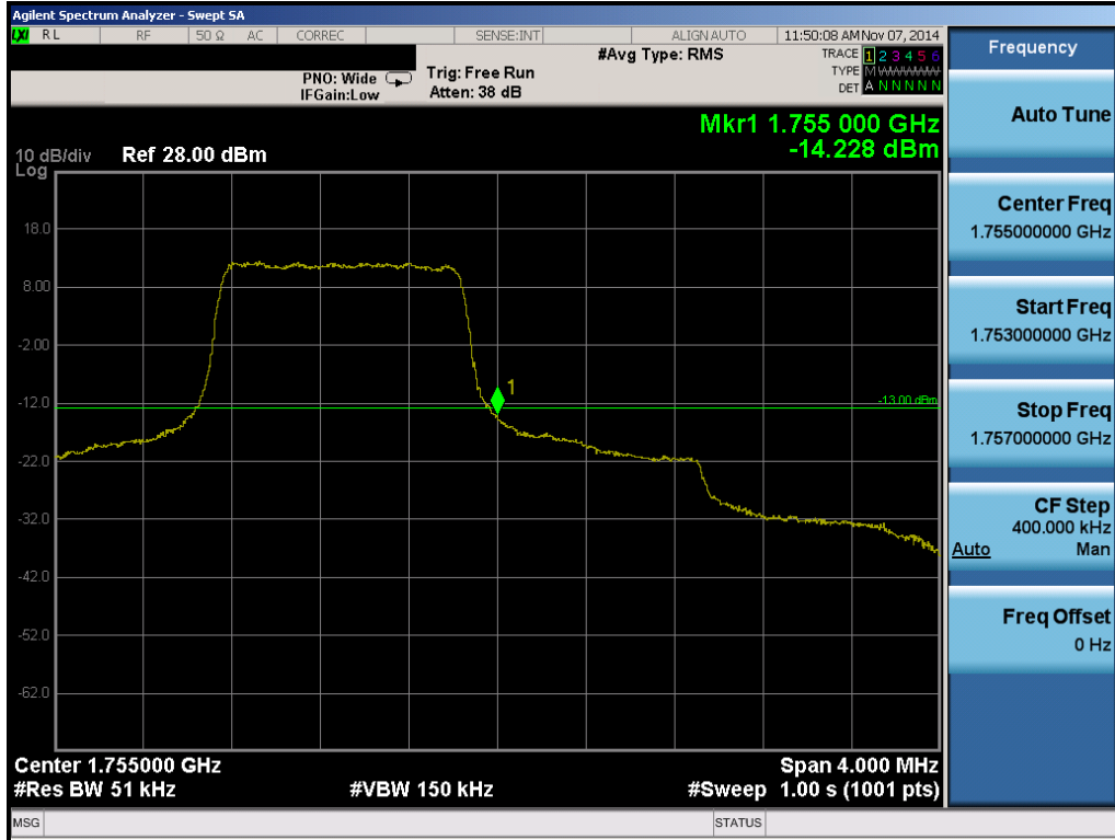
Plot 6-61. Upper Band Edge Plot (Band 4 – 1.4MHz QPSK – RB Size 6)
