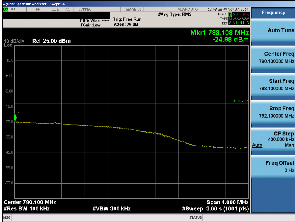
Plot 6-51. Upper Extended Band Edge Plot (Band 13 – 5.0MHz QPSK – RB Size 25)
