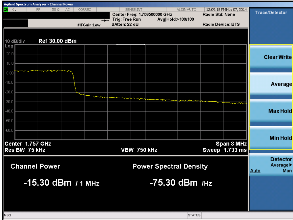
Plot 6-74. Upper Extended Band Edge Plot (Band 4 – 10.0MHz QPSK – RB Size 50)
