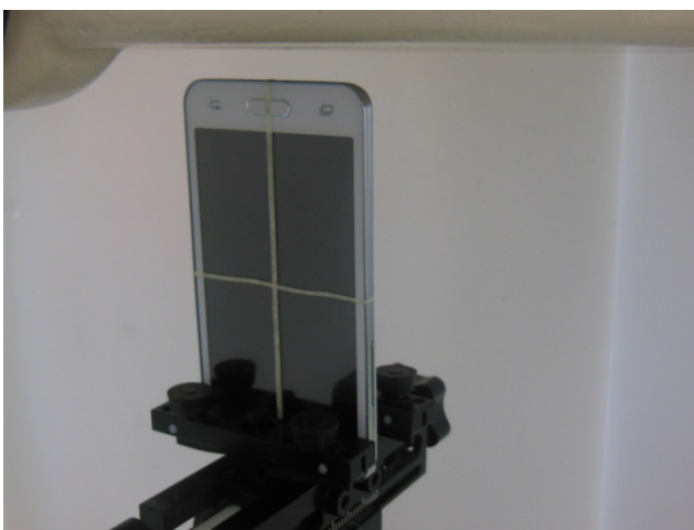
Bottom Side of the DUT with Phantom 1 cm Gap
