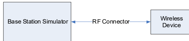
Figure 8-1 Power Measurement Setup
