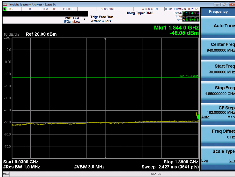
Plot 7-26. Conducted Spurious Plot (PCS WCDMA Mode – Ch. 9400)
