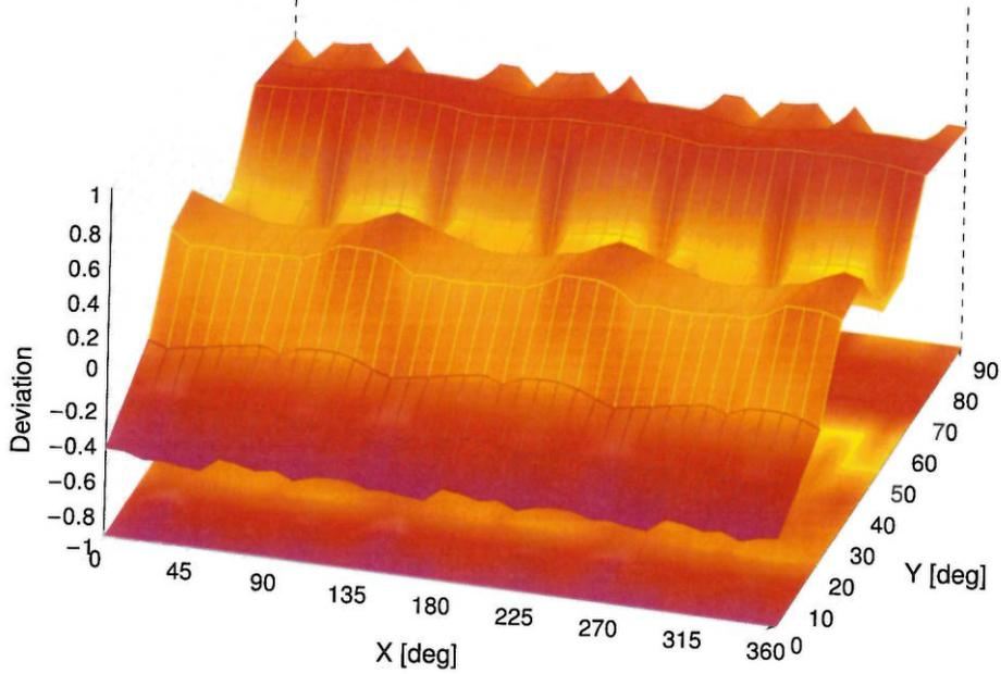
60GHz: 3D isotropy, E-field parallel to probe axis
