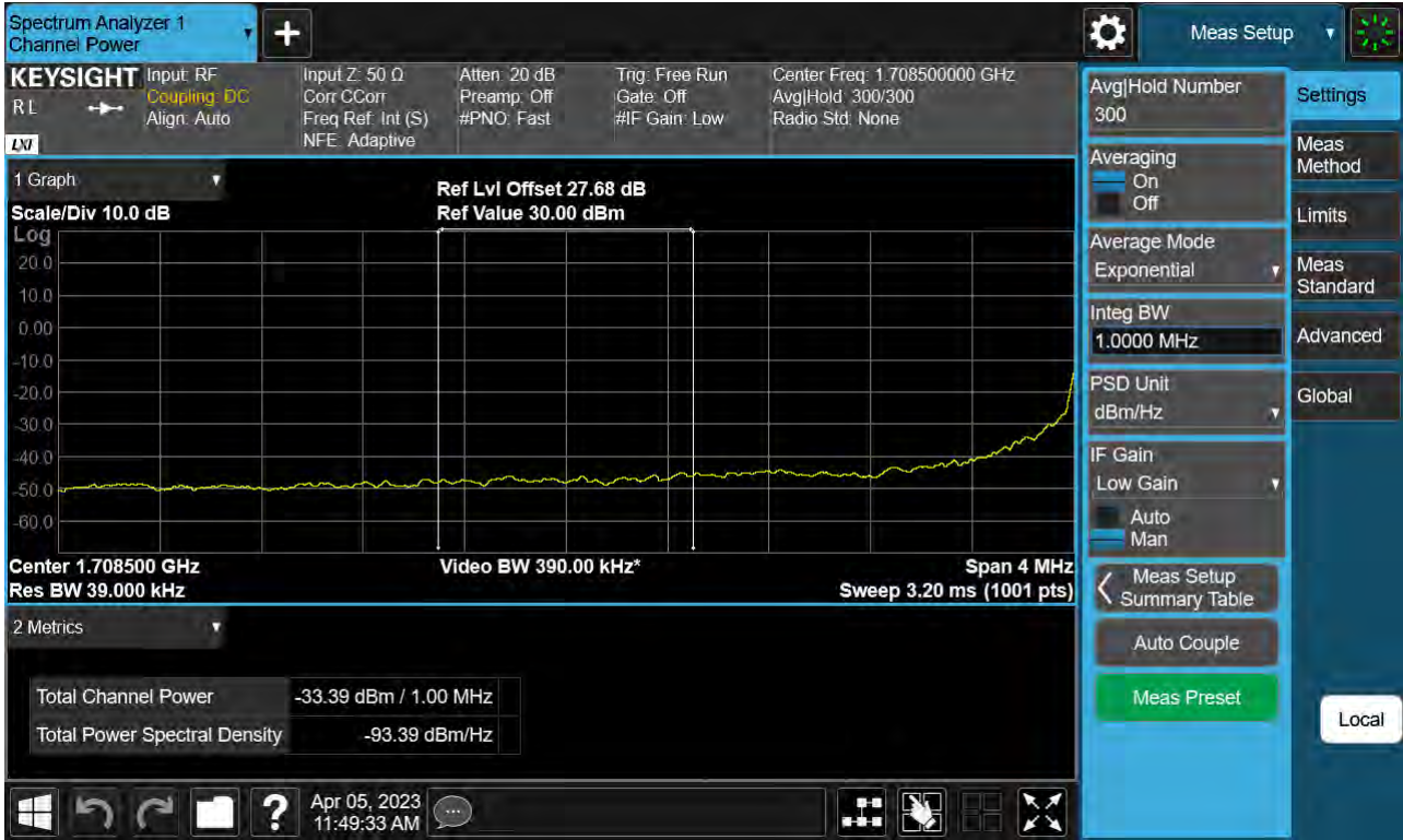
Sub6 n66. Lower Extended Band Edge Plot (25 M BW Ch.344500 BPSK_ Full RB) -3
