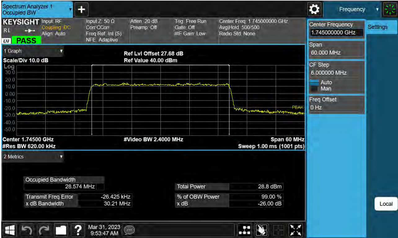
Sub6 n66. Occupied Bandwidth Plot (30 M BW Ch.349000 256QAM Full RB)
