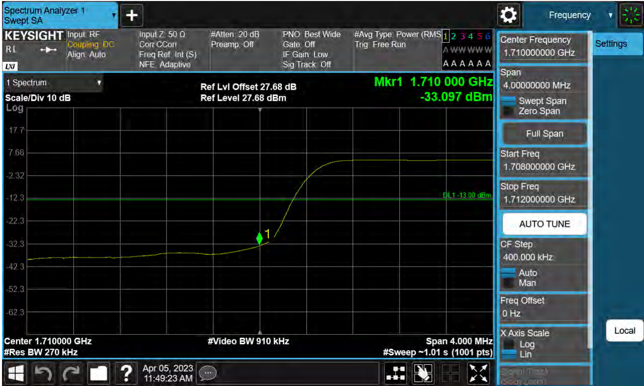
Sub6 n66. Lower Band Edge Plot (25 M BW Ch.344500 BPSK Full RB) -2
