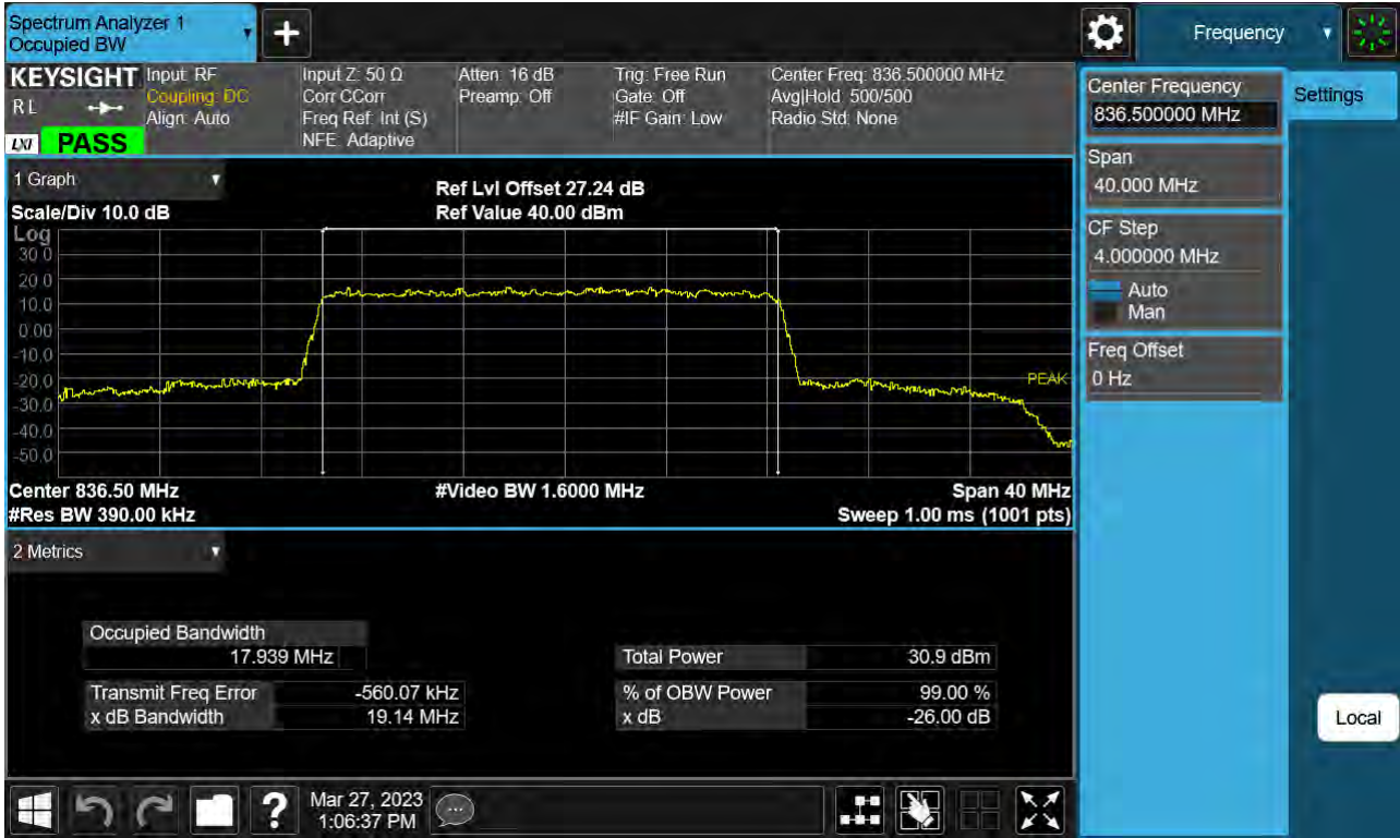
Sub6 n5. Occupied Bandwidth Plot (20 M BW Ch.167300 16QAM_ Full RB_0)
