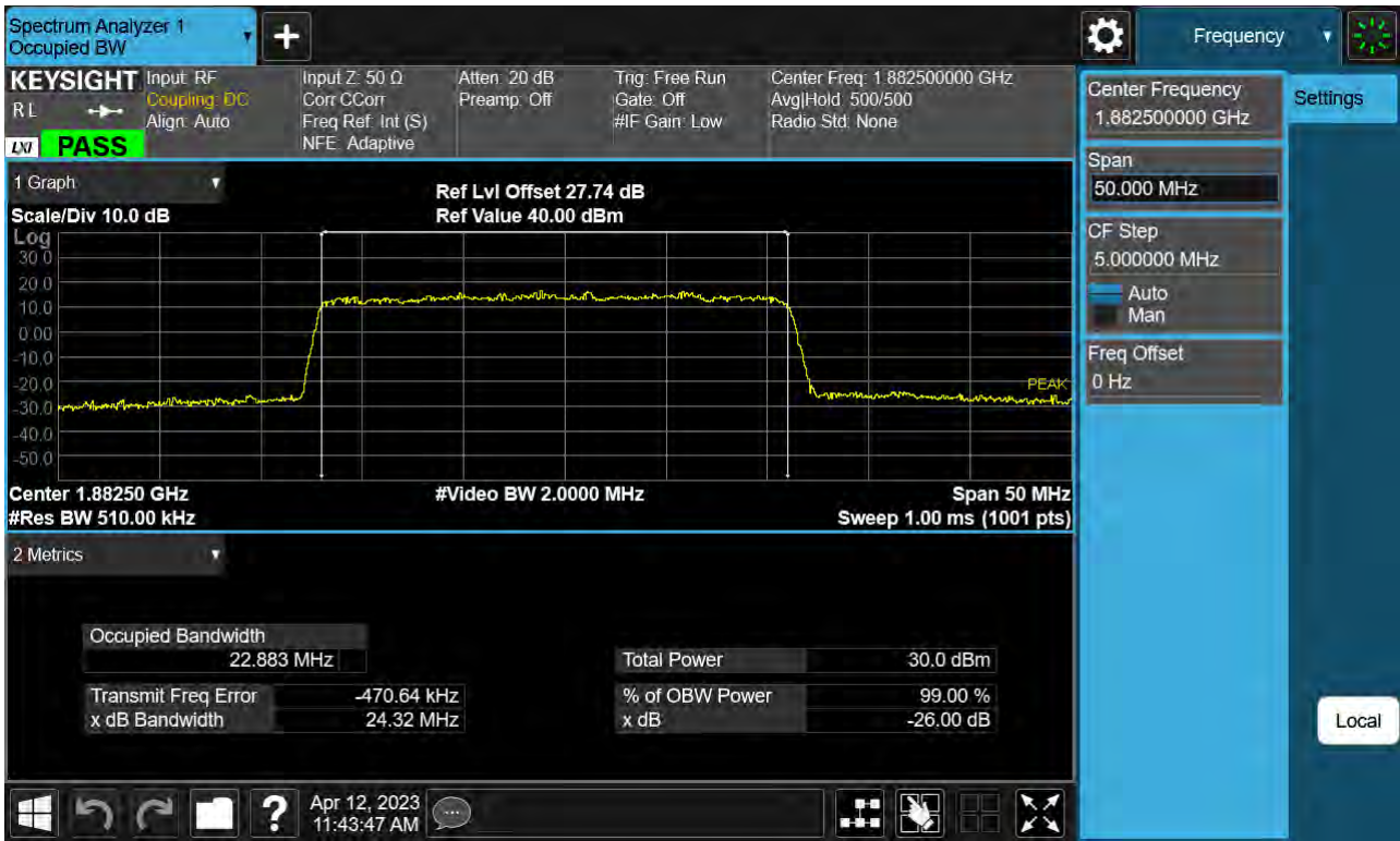
Sub6 n25. Occupied Bandwidth Plot (25 M BW Ch.376500 64QAM _ Full RB _0)
