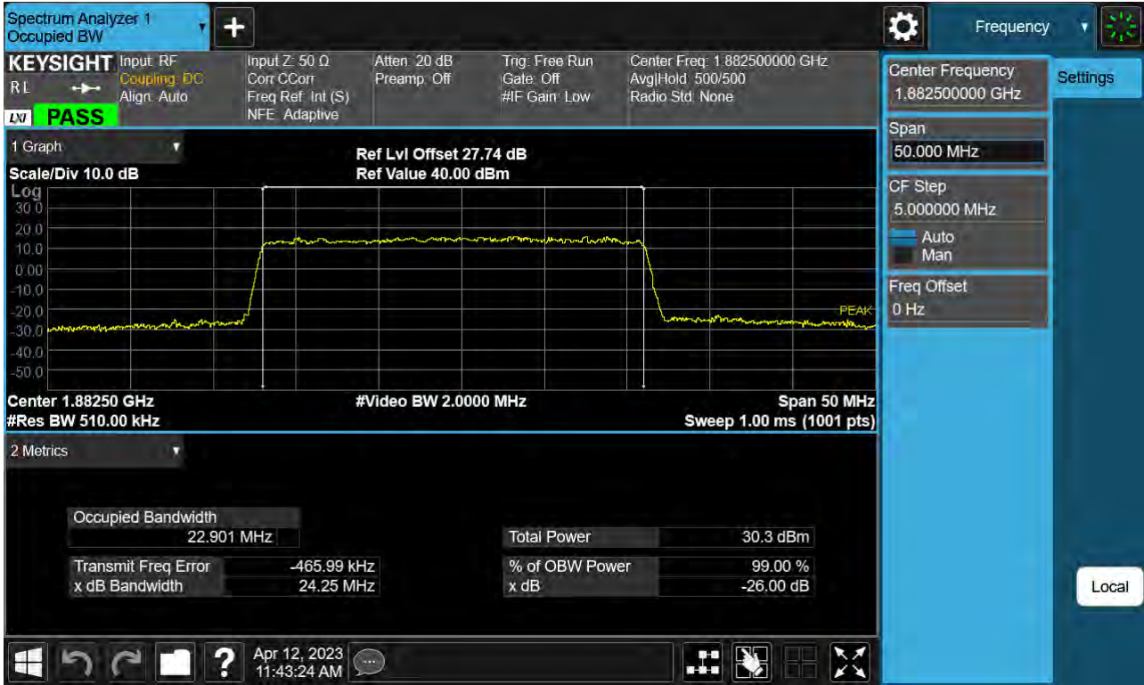
Sub6 n25. Occupied Bandwidth Plot (25 M BW Ch.376500 16QAM _ Full RB _0)
