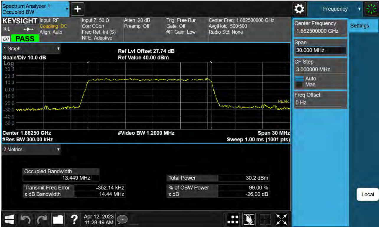
Sub6 n25(2). Occupied Bandwidth Plot (15 M BW Ch.376500 16QAM _ Full RB _0)
