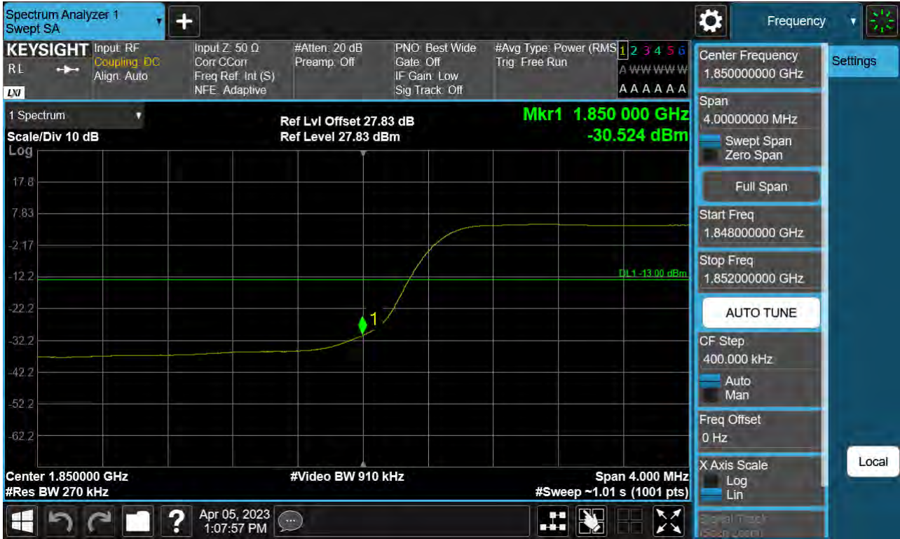
Sub6 n25. Lower Band Edge Plot (25 M BW Ch.372500 BPSK_RB100_Offset 0) -1
