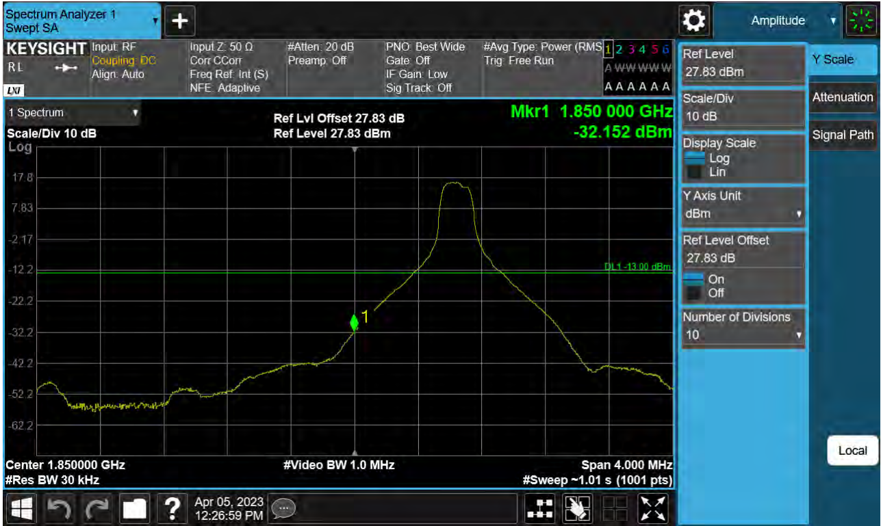
Sub6 n25. Lower Band Edge Plot (40 M BW Ch.374000 BPSK_RB1_Offset 0)
