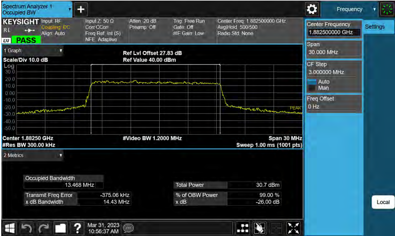
Sub6 n25(2). Occupied Bandwidth Plot (15 M BW Ch.376500 QPSK _ Full RB _0)
