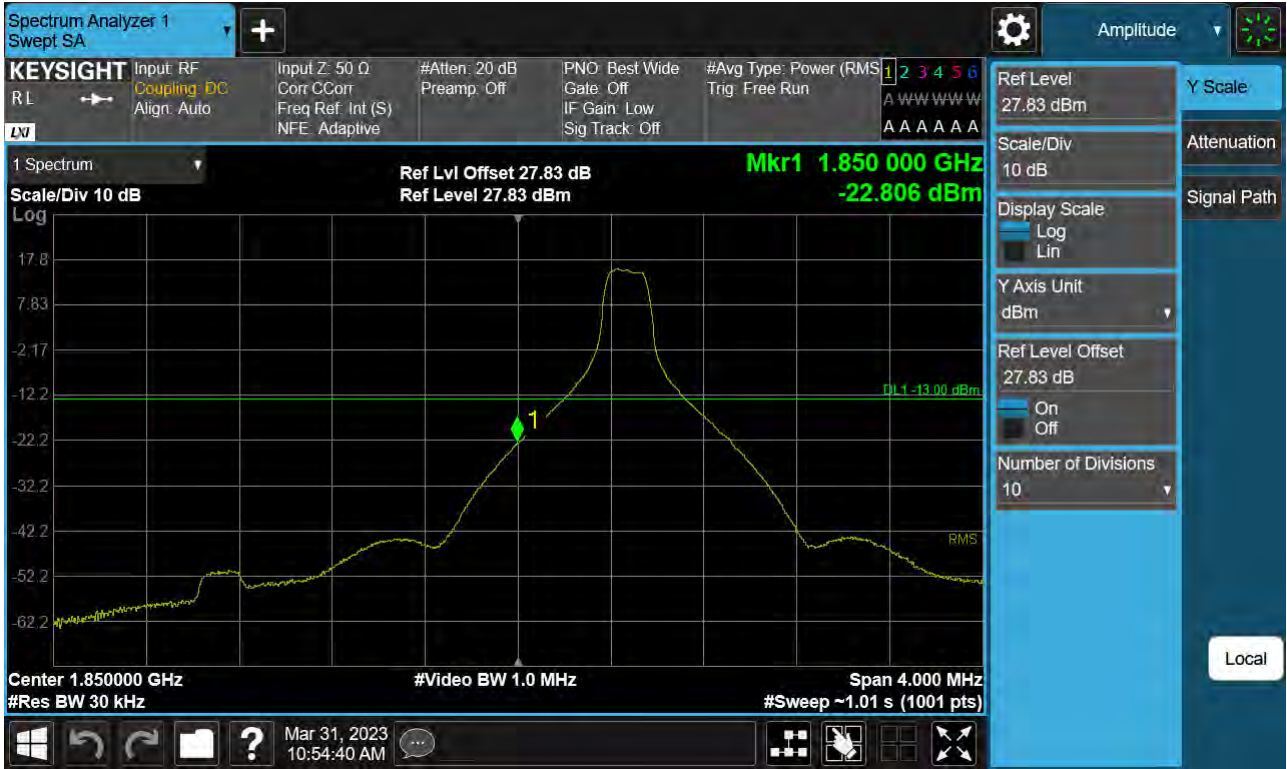
Sub6 n25(2). Lower Band Edge Plot (15 M BW Ch.371500 BPSK_RB1_Offset 0)
