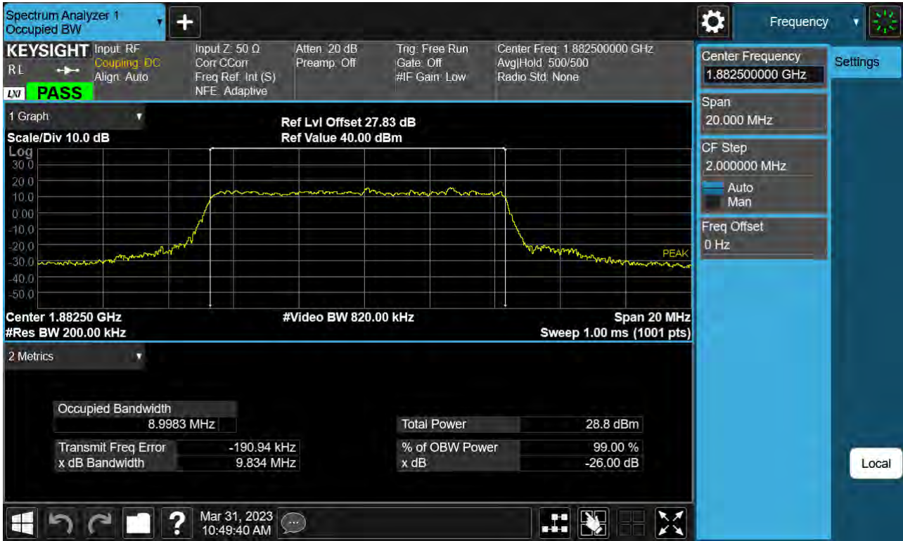
Sub6 n25(2). Occupied Bandwidth Plot (10 M BW Ch.376500 64QAM _ Full RB _0)
