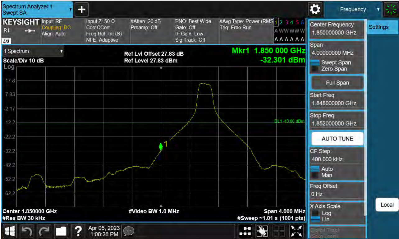
Sub6 n25. Lower Band Edge Plot (25 M BW Ch.372500 BPSK_RB1_Offset 0)
