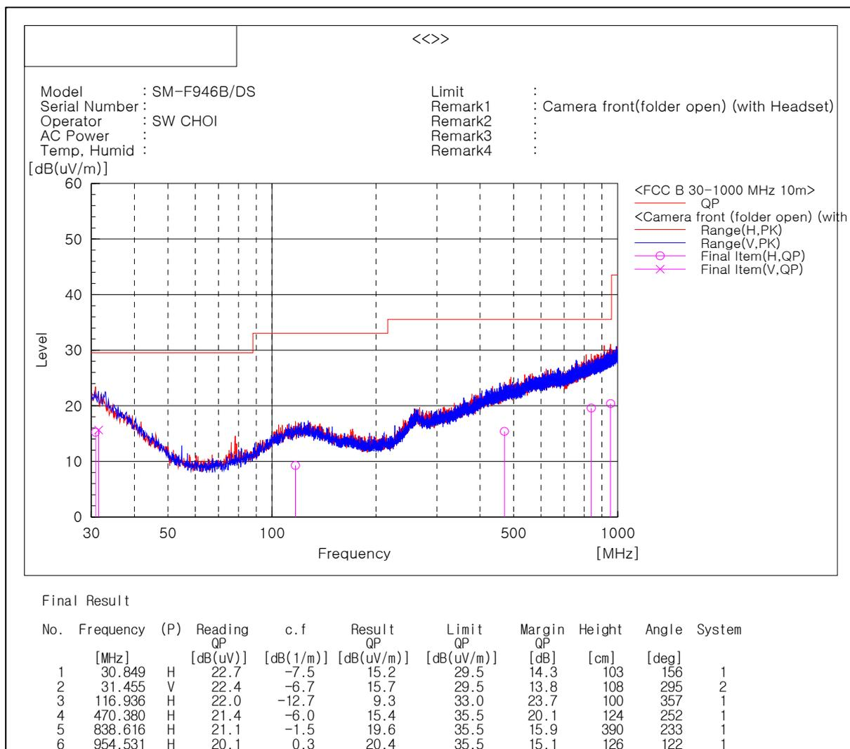
Note1) Receiving antenna polarization : Horizontal, Vertical
