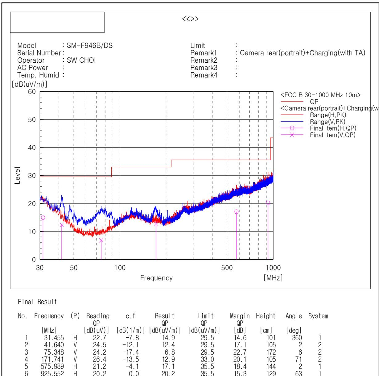
Note1) Receiving antenna polarization : Horizontal, Vertical
