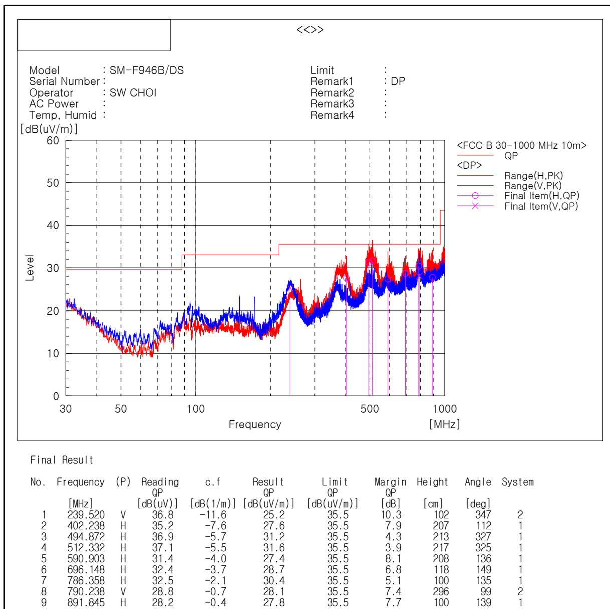
Note1) Receiving antenna polarization : Horizontal, Vertical
